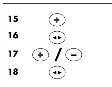
Press the + (15) button to display the next program item **P03**, the automatic shower function switch-off time. The value 15 min. is displayed when the **MODE (16)** button is pressed. Use the +/- (17) buttons to adjust this value within the range 1 to 50 minutes. Store this setting with the **MODE (18)** button. The display shows **P03**.
