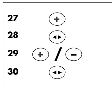
Press the + (27) button to display the next program item **P07**, the characteristic curve. The value 1 is displayed when the **MODE (28)** button is pressed. Use the +/- (29) buttons to set the value 0 (No) or 1 (Yes). Store this setting with the **MODE (30)** button. The display shows **P07**.
