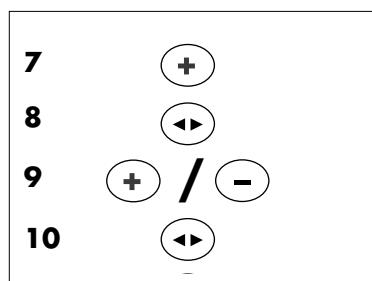
Press the **+** (7) button to display the next program item **P01**, the lower reset limit. The value 32°C is displayed when the **MODE** (8) button is pressed. Use the **+/-** (9) buttons to adjust this value within the range 10°C to 32°C. Store this setting with the **MODE** (10) button. The display shows **P01**.
