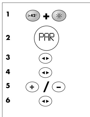
To display the program menu, press the **>42° + Shower lighting** (1) buttons at the same time for at least 5 seconds until **P00** (2) is displayed. Press the **MODE** (3) button. **P00**, the program item for the upper reset limit, is shown on the display. The value 42°C is displayed when the **MODE** (4) button is pressed again. Use the **+/-** (5) buttons to adjust this value within the range 32°C to 42°C. Store this setting with the **MODE** (6) button. The display shows **P00**.
