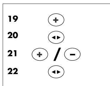
Press the + (19) button to display the next program item **P04**, automatic lighting switch-off. The value 2 is displayed when the **MODE (20)** button is pressed. Use the +/- (21) buttons to adjust this value within the range 1 to 50 minutes. Store this setting with the **MODE (22)** button. The display shows **P04**.
