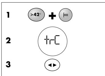
Press the **>42° + Hydromassage (1)** buttons at the same time for at least 5 seconds until trC (2) is displayed. (Press the **>42°** button again if you wish to interrupt this process.) Now press the **MODE (3)** button: The reset is performed.
