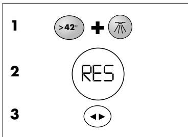
Press the **>42° + Overhead shower (1)** buttons at the same time for at least 5 seconds until RES (2) is displayed. (Press the **>42°** button again if you wish to interrupt this process.) Now press the **MODE (3)** button: The reset is performed.
