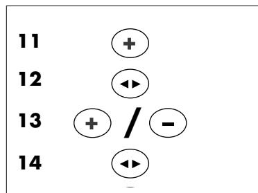
Press the **+** (11) button to display the next program item **P02**, the upper setting limit of the shower temperature. The value 55°C is displayed when the **MODE** (12) button is pressed. Use the **+/-** (13) buttons to adjust this value within the range 40°C to 60°C. Store this setting with the **MODE** (14) button. The display shows **P02**.
