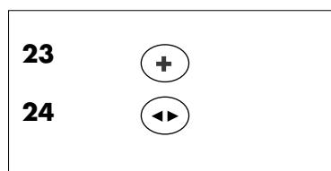
Press the + (23) button to display the next program item **P05**, the configuration code. A three-digit configuration code is displayed when the **MODE (24)** button is pressed.
