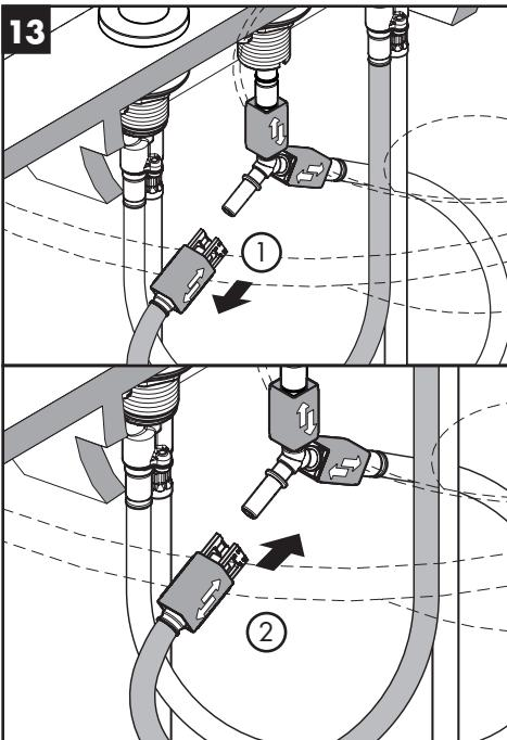
Open the quick-connect on one of the connection hoses by pushing it upwards.
