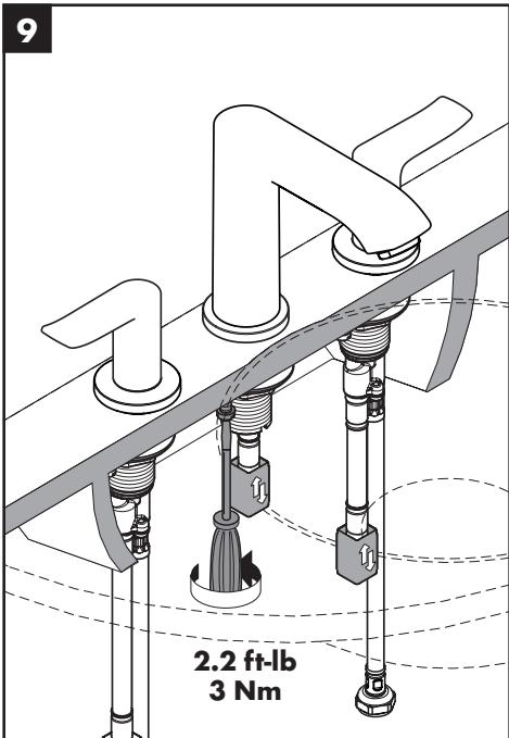
Tighten the tensioning screws.
