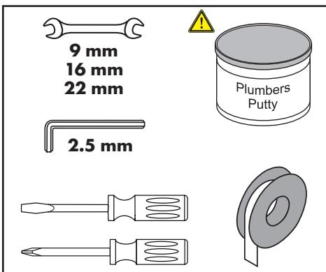
⚠ Petroleum-based plumbers putty can damage the surface of some sinks. Please consult the manufacturer of the sink regarding compatible sealants.
