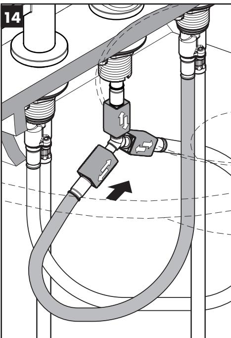
Lock the quick-connect by pushing it toward the connection angle.
