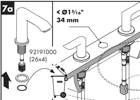
If the hole for the spout is less than 1 5/16" (34 mm), discard the 26x4 o-ring. Install the gasket on the spout.
