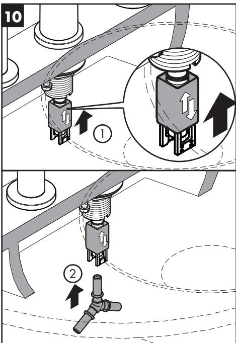
Open the quick-connect by pushing it upwards.
