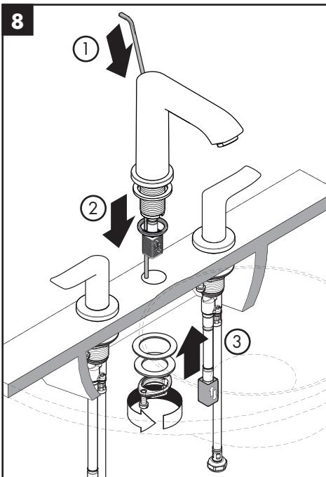
Install the drain pull rod on the spout.
