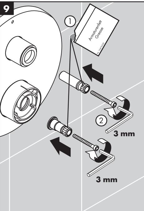
Lubricate the adapter stems with a small amount of white plumber's grease.
