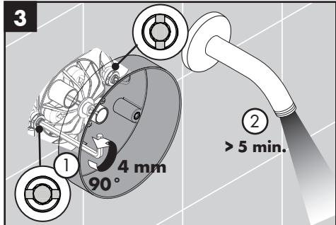
Open the hot stop. Allow the hot supply to flush for at least 5 minutes.
