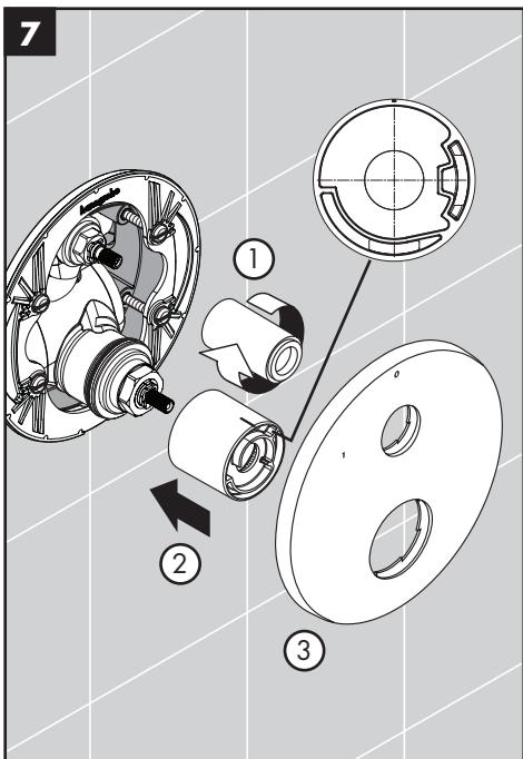
Slide the thermostatic mixer sleeve on so that the indexing mark is at the 12:00 position.
