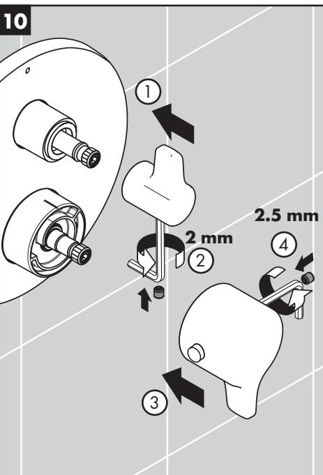
Install the volume control handle. Tighten the screw using a 2 mm Allen wrench. Install the screw cover.
