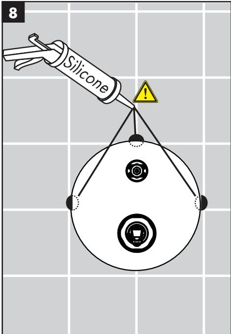
Place a dab of waterproof sealant at each grout joint.
