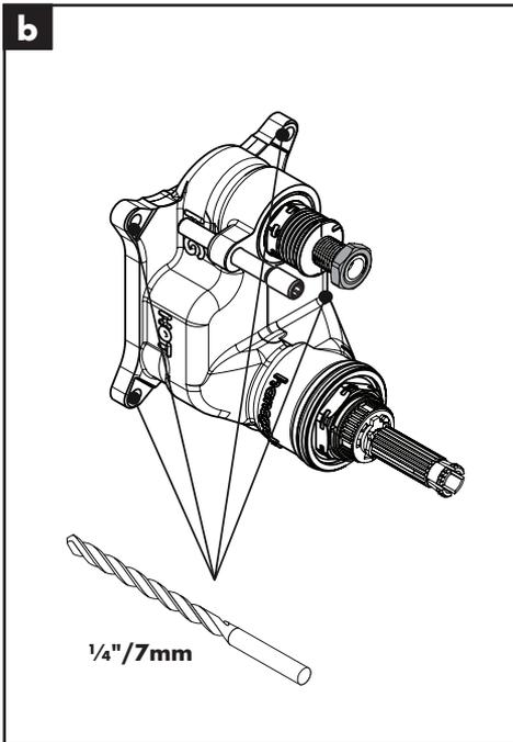
Use a 1/4" drill bit to slightly enlarge the screw holes on the function block.
