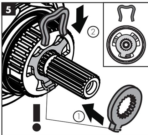
\*\*Follow all applicable local plumbing codes when setting the high temperature limit stop. To prevent scald injury, the maximum output temperature of the shower valve must be no higher than 120°F (49°C). In Massachusetts, the maximum output temperature can be no higher than 112°F (44°C).
