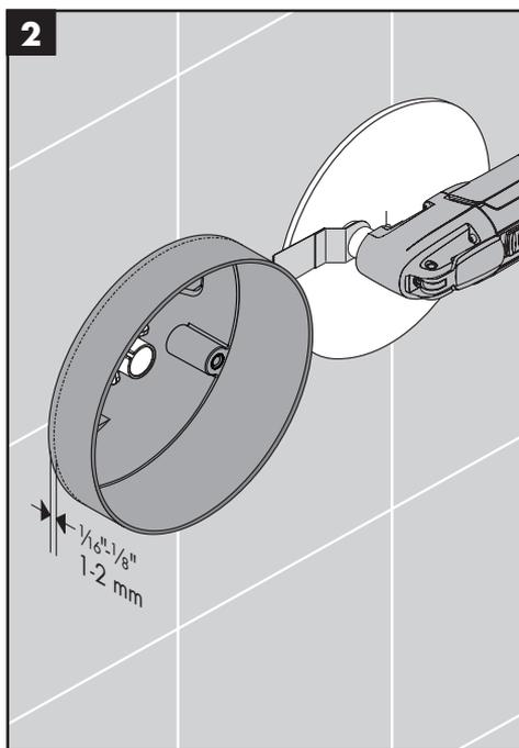
Cut the plaster shield so that it extends  $\frac{1}{16}$ "- $\frac{1}{8}$ " (1-2 mm) outside the surface of the finished wall.
