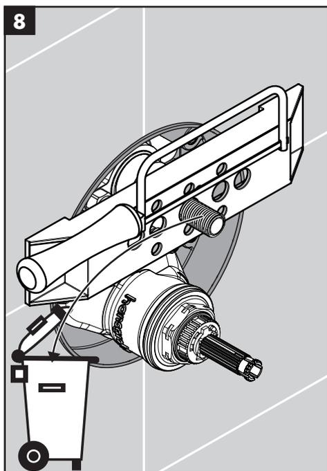
Cut the shutoff stem so that it is even with the front of the fitting aid.
