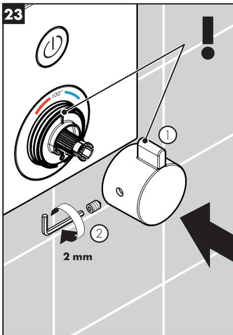
Install the handle so that the lever is next to the indexing mark on the sleeve and the 100° marking on the escutcheon.
