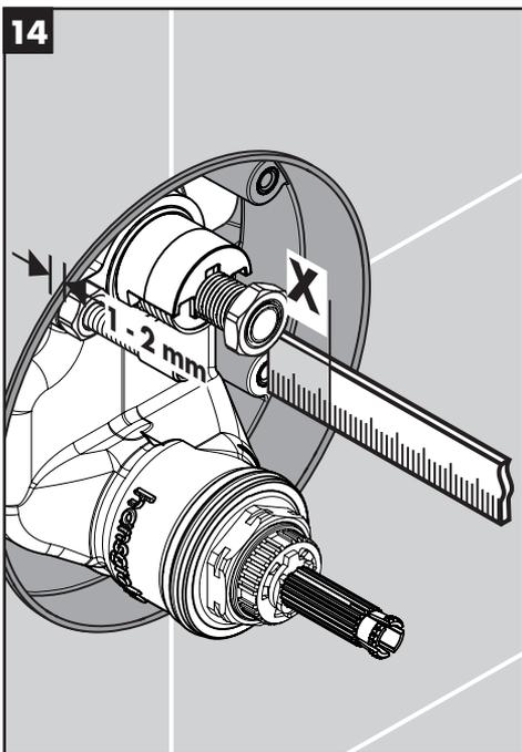
Measure the distance between the outside edge of the plaster shield and the screw flange (X).
