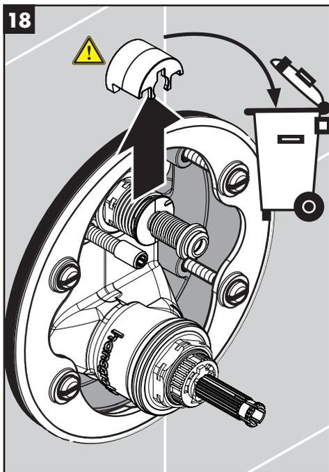
**IMPORTANT:** Remove the safety guard from the shutoff valve.
