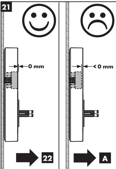
In the "off" position, the front of the shutoff button should be flush with the front of the escutcheon.
