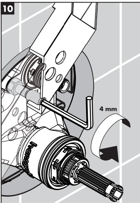
Raise the spacer so that it is even with the back of the fitting aid.
