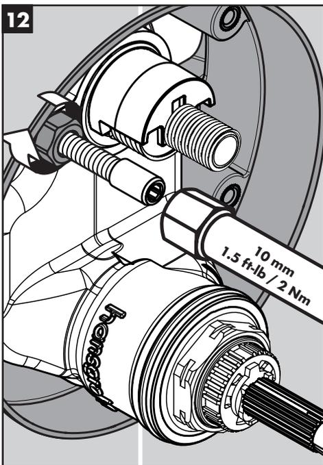
Tighten the nut on the spacer.
