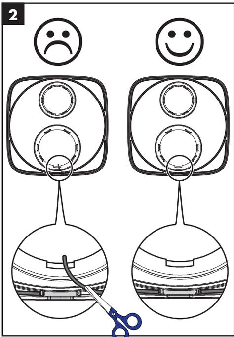
The gasket should not go into the notch on the bottom of the escutcheon.
