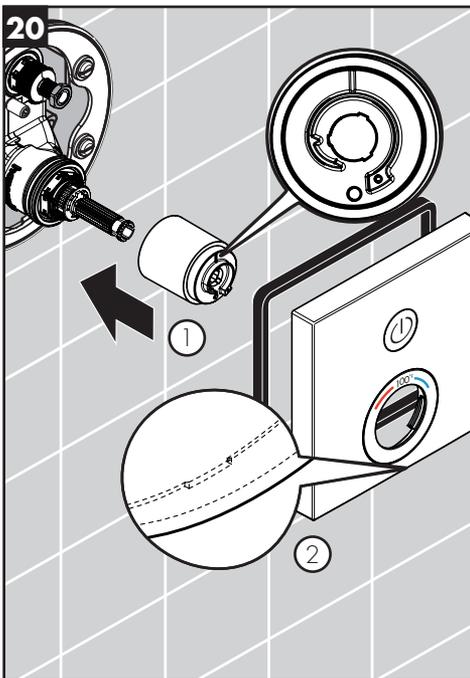
Install the thermostatic mixer sleeve.
