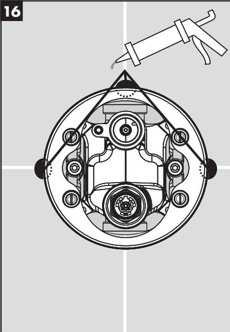
Place a small amount of caulk at the top and side joint joints.
