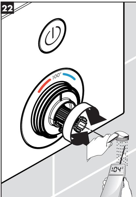
Turn the thermostatic mixer stem until the output water is 104°F (40°C).
