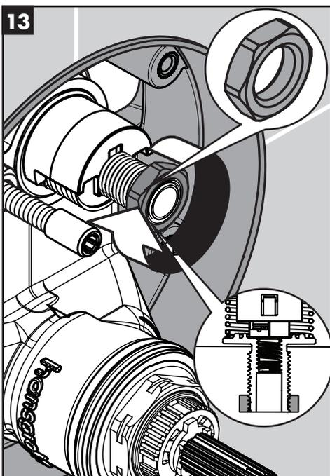
Install the nut on the shutoff valve stem so that it is even with the front of the stem.
