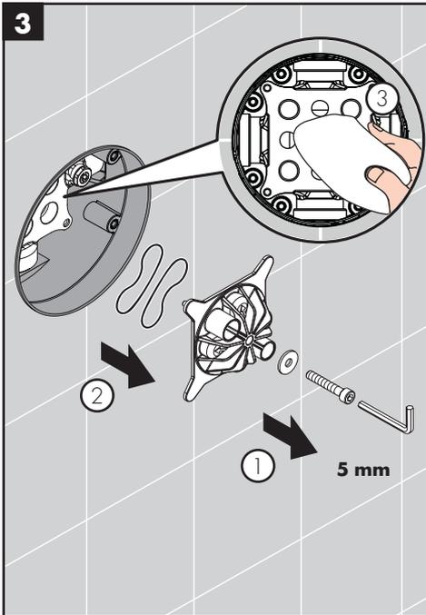
Remove the flush insert and the flush insert seals.
