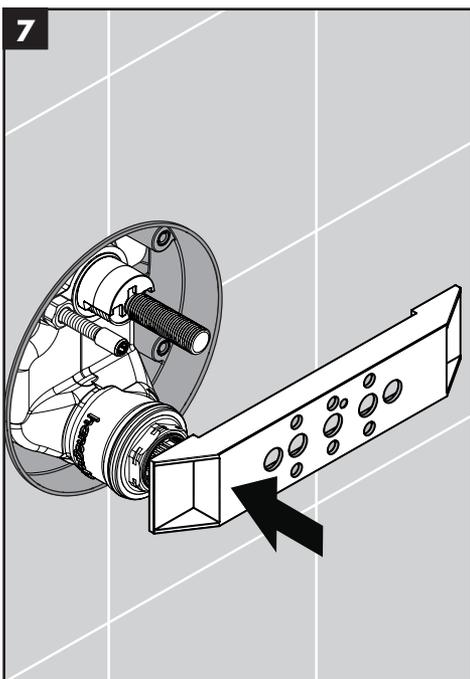
Position the fitting aid over the shutoff stem.
