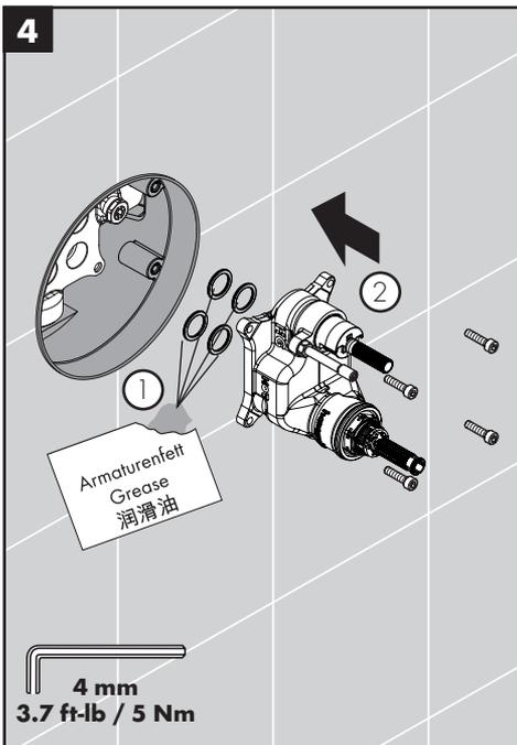
Lightly lubricate the function block o-rings.
