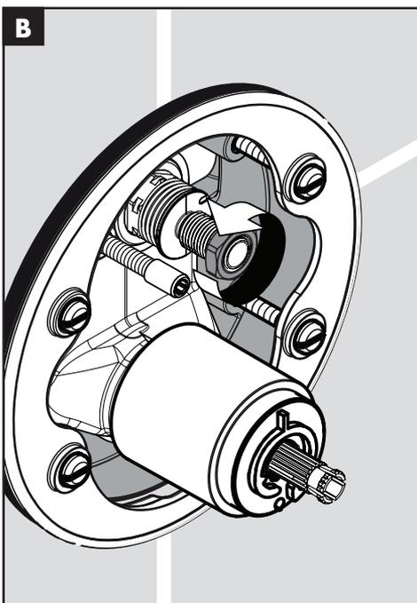
Rotate the nut on the shutoff stem slightly counter-clockwise, to bring it out farther.
