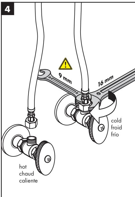
Connect the hoses to the stops. Use two wrenches, as shown in the diagram.
