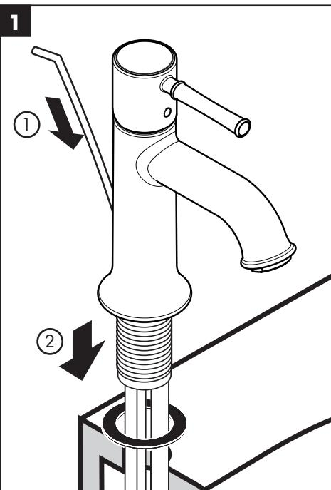
Install the drain pull rod on the faucet.
