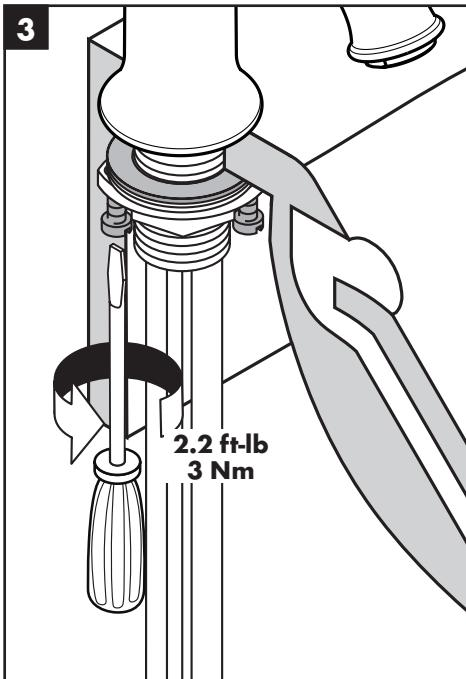
Tighten the tensioning screws.
