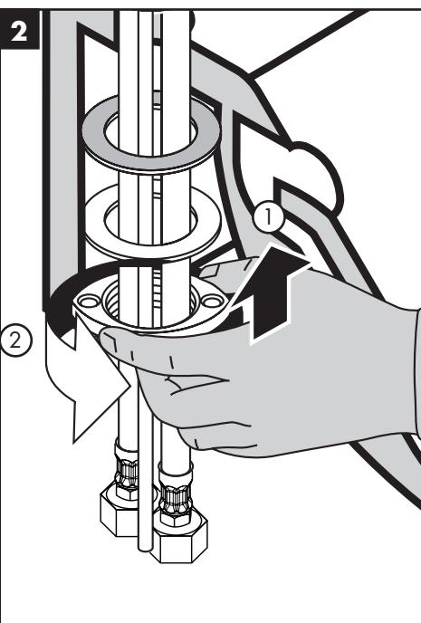
Install the fiber washer, friction washer and mounting nut.
