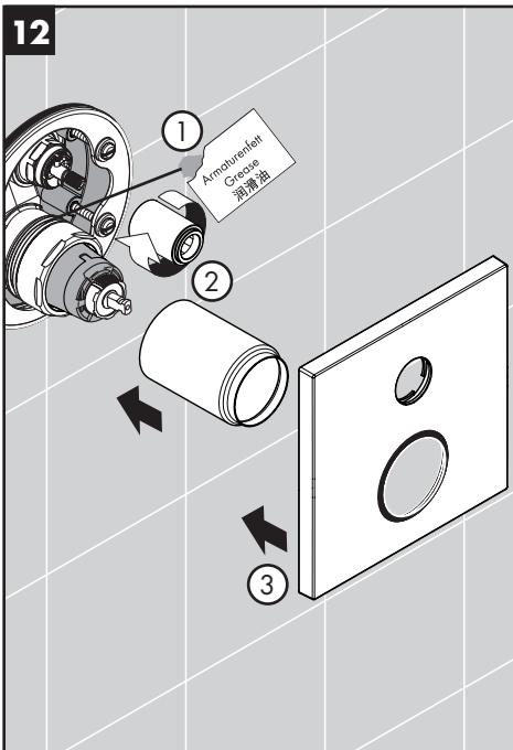
Lubricate the pressure balance cartridge o-ring using a small amount of white plumber's grease.
