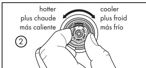
Rotate clockwise to decrease the maximum temperature. Rotate counter-clockwise to increase the maximum temperature.
