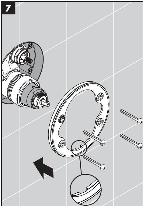
Install the carrier plate so that the notch is at the bottom.
