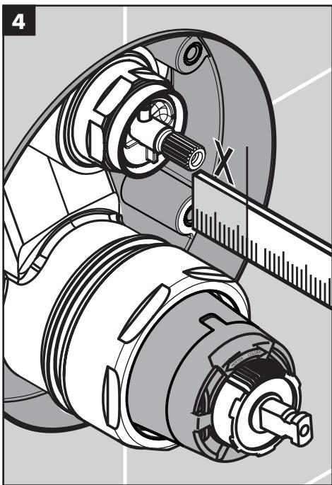
Measure the distance from the front of the plaster shield to one of the screw-in flanges ("X").
