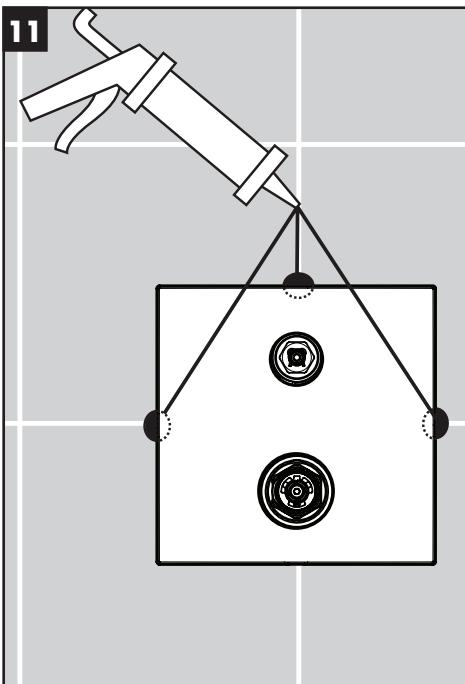
Place a small amount of caulk at the top and side grout lines where the escutcheon will rest.
