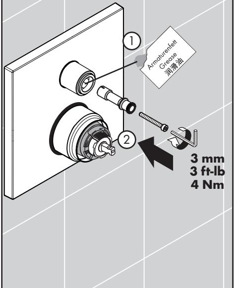
Lubricate the diverter stem with a small amount of white plumber's grease.
