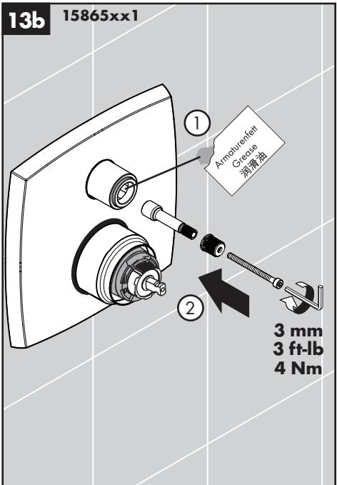
**15865xx1 only:** Install the handle adapter and the snap connector. Tighten the screw.
