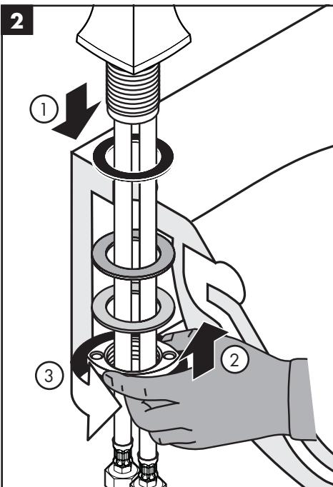
Position the faucet and sealing ring on the mounting surface.
