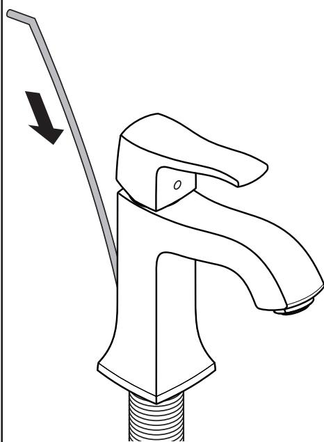
Install the drain pull rod on the faucet.
