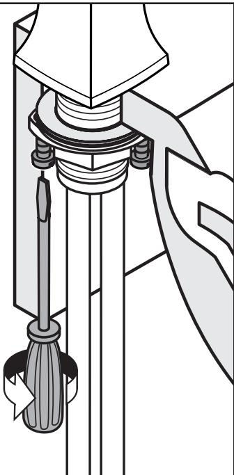
Tighten the tensioning screws.
