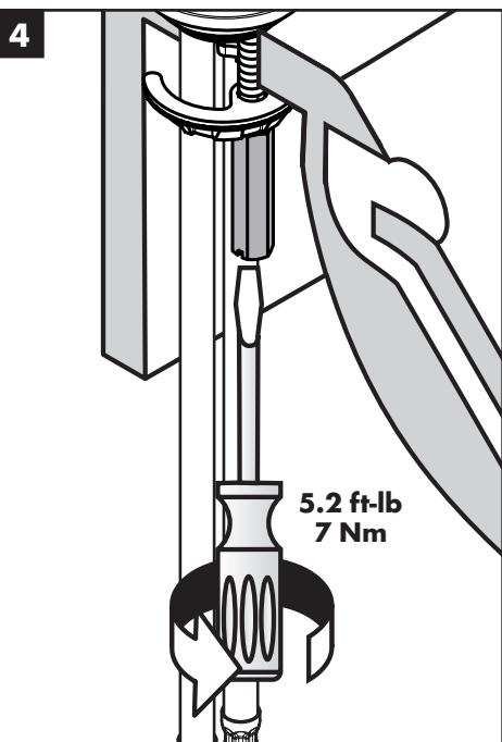
Tighten the collar using a flat head screwdriver.
