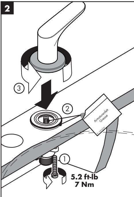
Tighten the tensioning screws.
