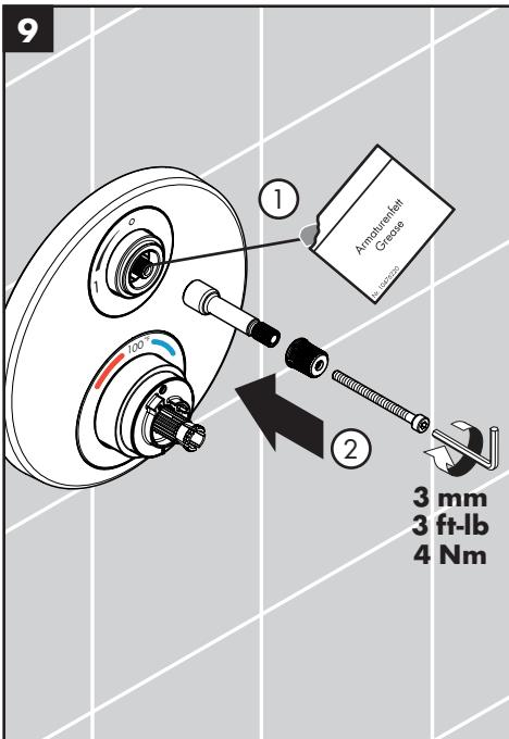
Lubricate the volume control stem with a small amount of white plumber's grease.
