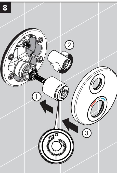
Slide the thermostatic mixer sleeve on so that the indexing mark is at the 12:00 position.
