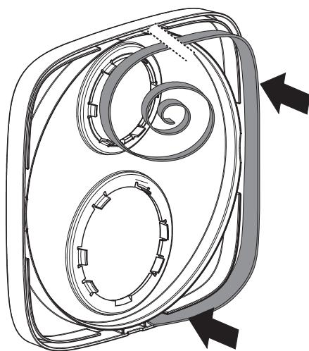
**Square and SoftCube escutcheons only:** Push the flexible sealing gasket into the channel on the rear of the escutcheon.
