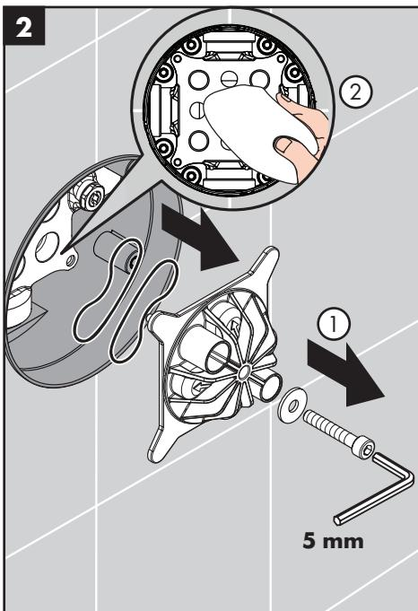
Remove the flush insert and the flush insert seals.
