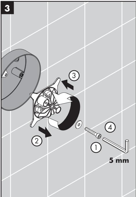
Use a 5 mm Allen wrench to remove the flush insert. Turn it 90° and reinstall it.
