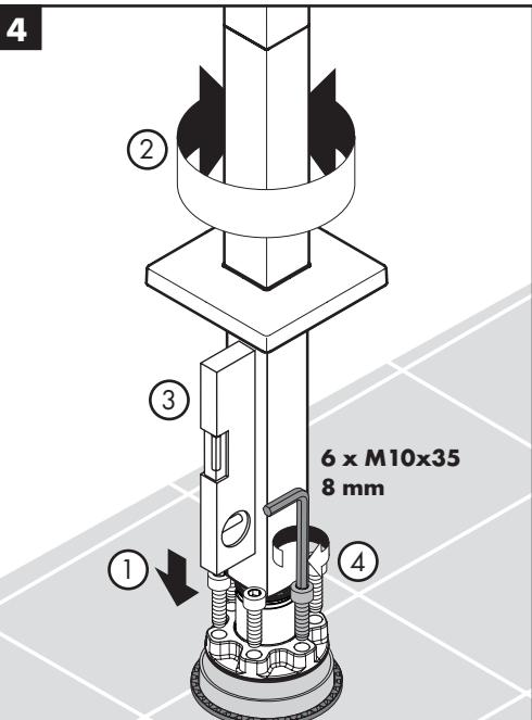
Position the tub spout over the rough. Rotate the spout to the correct position.
