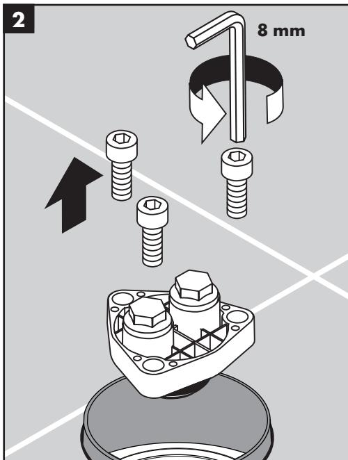
Remove the flush insert.
