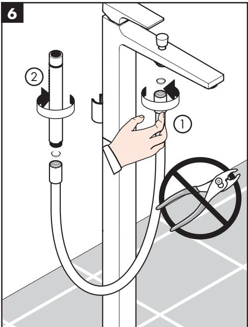
**⚠ Do not use pliers to tighten the hose nuts as they will damage the finish.**
