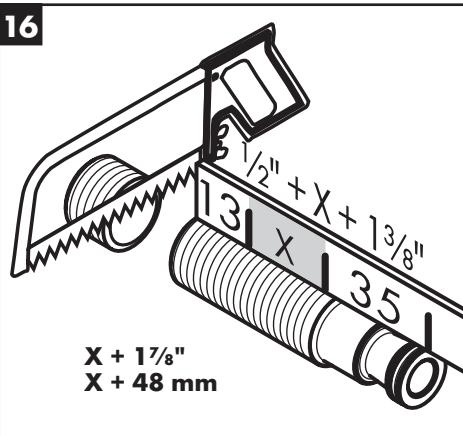
Cut the threaded portion of the spout so that it is  $X + 1\frac{7}{8}$ " ( $X + 48$  mm) long.
