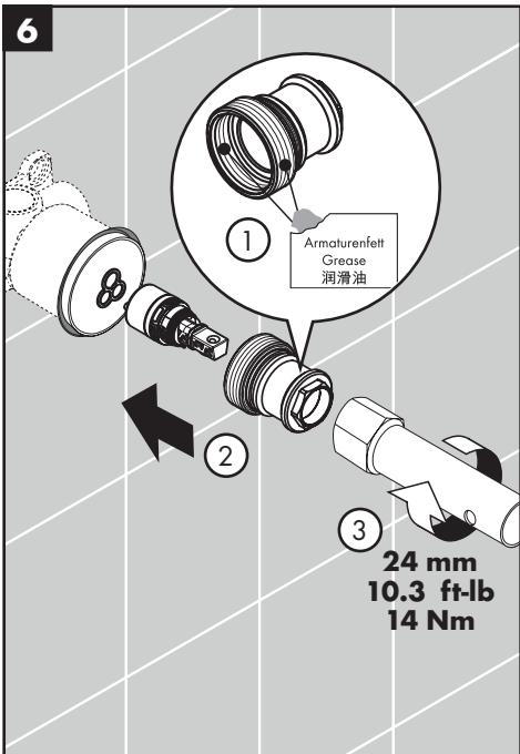
Lightly lubricate the threads on the nut.
