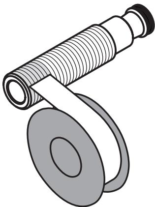
Wrap the threads with several layers of plumbers' tape.
