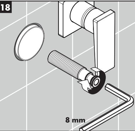
Install the connecting thread in the rough.
