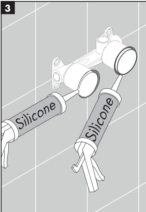
Seal the wall around the plaster shields using water-proof sealant.
