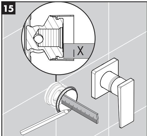
Measure the distance from the surface of the spout port rough to the outside edge of the plaster shield ("X").
