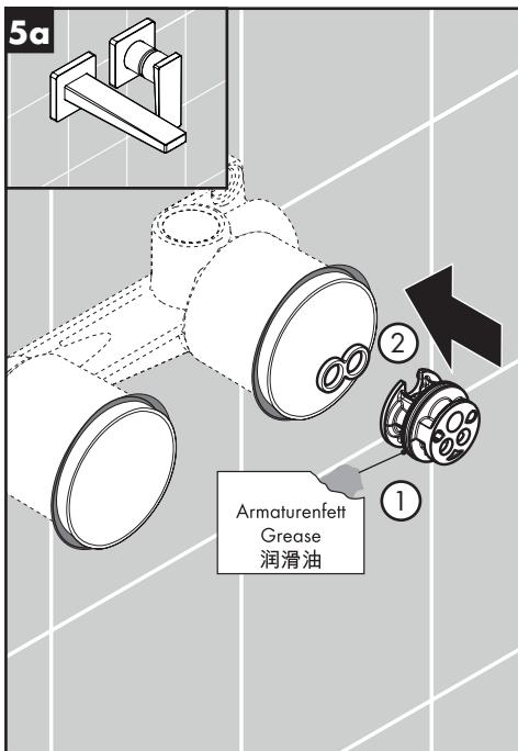
Lightly grease the o-ring on the cartridge adapter.
