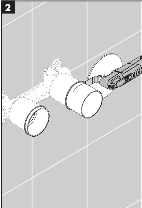
Cut the plaster shields so that they extend  $\frac{1}{16}$ " (1mm) outside the surface of the finished wall.
