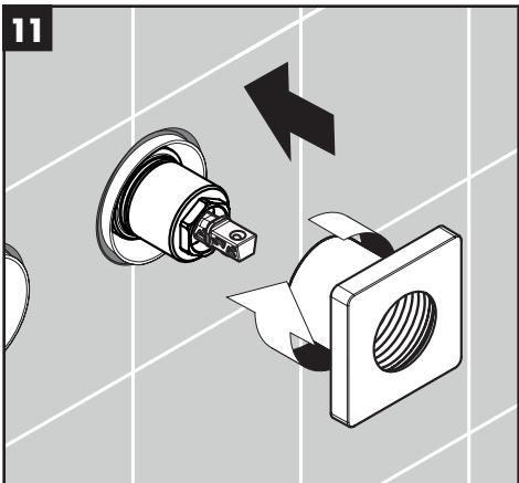
Install the sleeve/escutcheon assembly over the cartridge.
