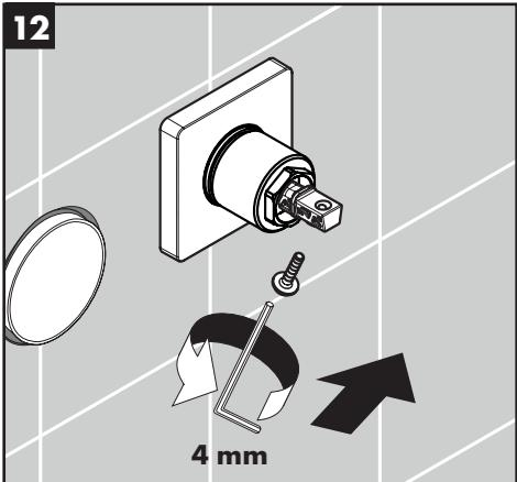
Install the handle screw on the cartridge stem.
