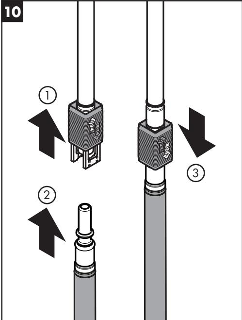
Push the quickconnect barb into the coupling hose and slide the retainer sleeve down until it clicks.
