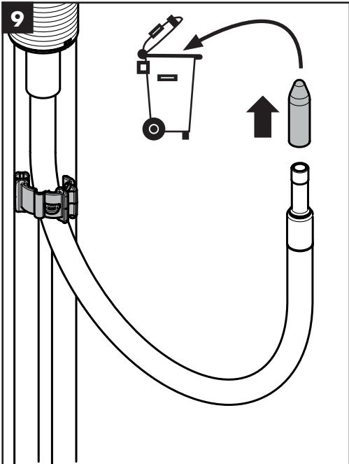
Remove the protective cap from the quickconnect barb at the end of the pullout hose and discard.
