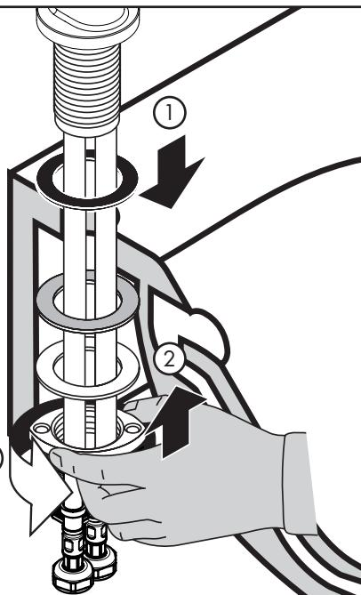
Place the fiber washer, then the friction washer and then the mounting nut onto the faucet.
