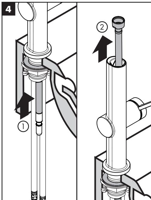
Push up on the pullout sprayer hose from the bottom of the faucet and remove some hose slack from the top.
