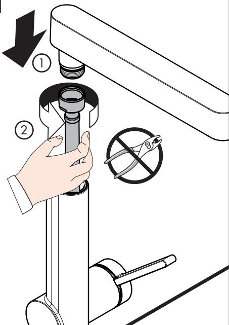
Press the spout connection into the pullout hose and tighten the hose nut by hand
