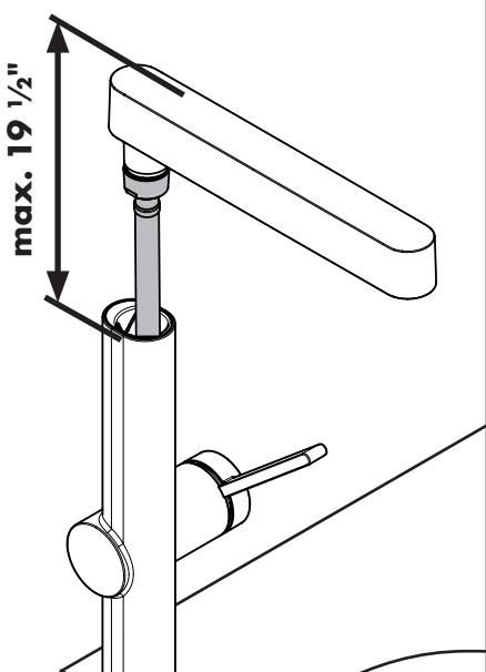
Pull up on the spout a maximum of 19 1/2" and carefully set it down on a towel or other soft surface.
