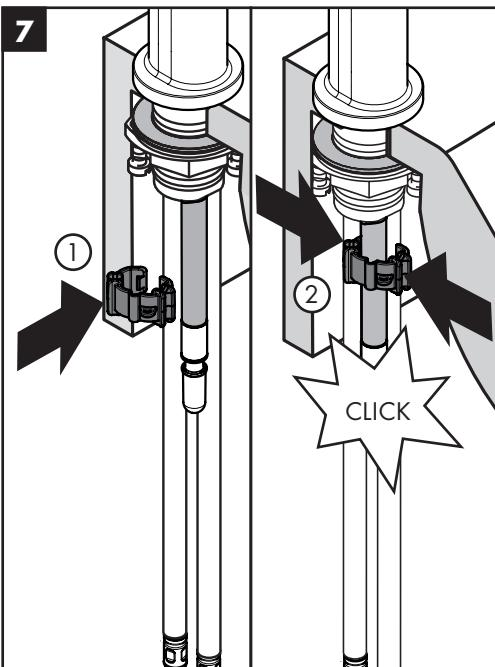
Snap the retainer clip onto the remaining pullout hose on the underside of the faucet the to limit the maximum pullout length.
