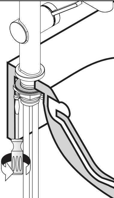
Tighten the tensioning screws.
