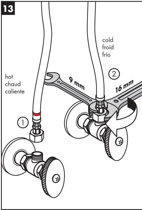
Connect the hot and cold supply hoses to the stops.
