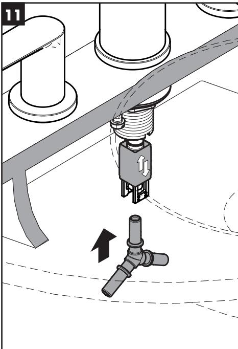
Insert the connection angle in the spout quick-connect.
