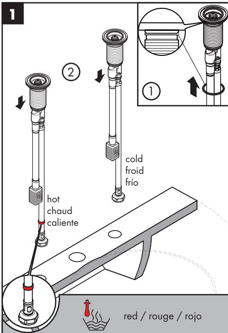
Install the 26x2.5 centering o-ring on each valve.
