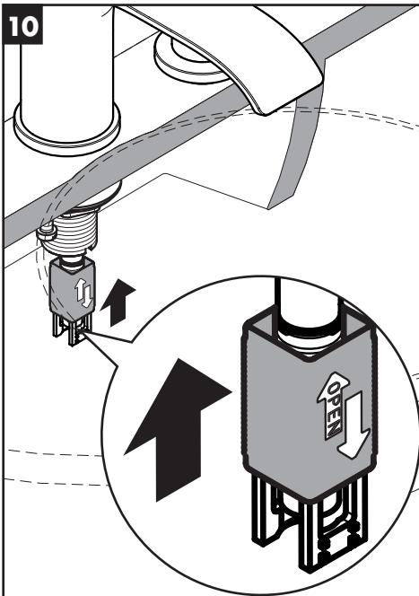
Open the quick-connect by pushing it upwards.
