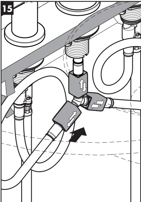
Lock the quick-connect by pushing it toward the connection angle.
