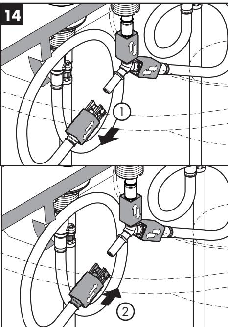
Open the quick-connect on one of the connection hoses by pushing it upwards.
