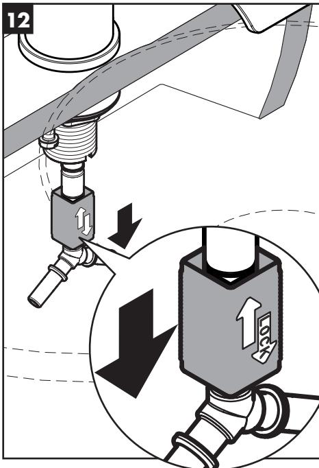
Lock the quick-connect by pulling down on it.
