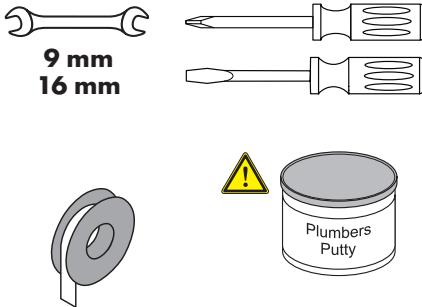
⚠ **WARNING:** Petroleum-based plumbers putty can damage the surface of some sinks. Please consult the manufacturer of the sink regarding compatible sealants.
