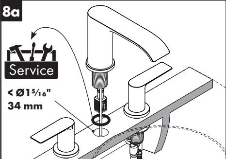
If the hole for the spout is less than  $1\frac{5}{16}$ " (34 mm), discard the 26x4 o-ring.
