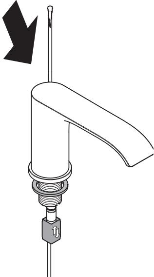
Install the drain pull rod on the spout.
