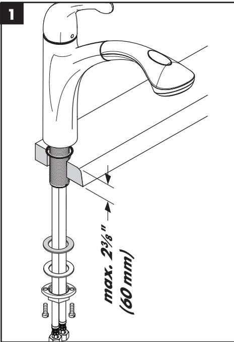
Place the faucet and sealing ring on the mounting surface.
