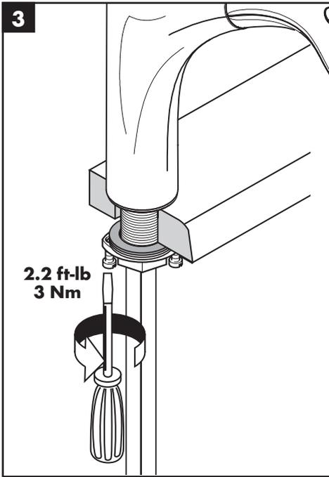
Tighten the mounting nut.
