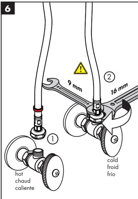
Connect the hot and cold supply hoses to the stops.
