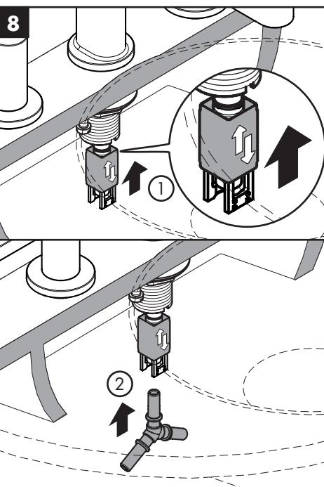
Open the quick-connect by pushing it upwards.
