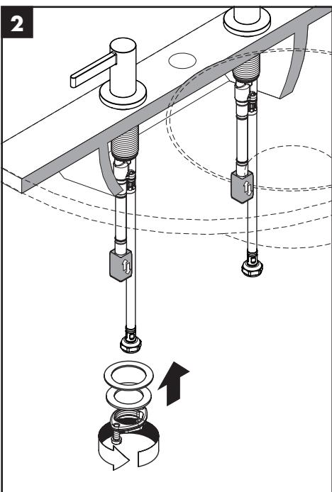
Install the fiber washer, metal washer, and mounting nut.
