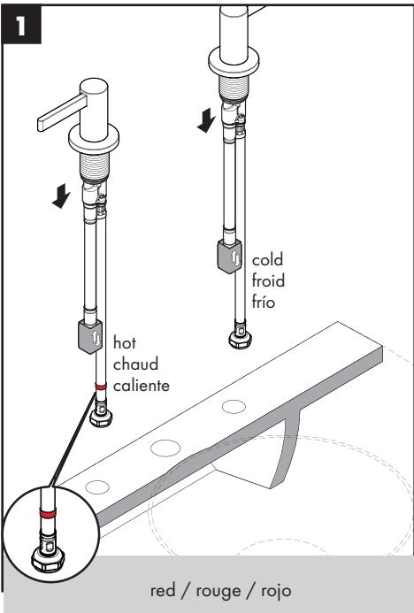
Place the hot and cold valve assemblies on the mounting surface. The hot valve should be on the left, the cold valve on the right.
