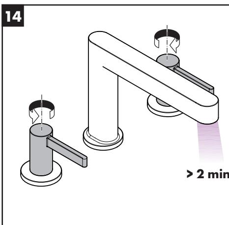
Flush the hot and cold supply lines for at least two minutes.
