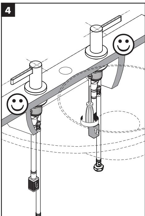
If necessary, rotate the valve.
