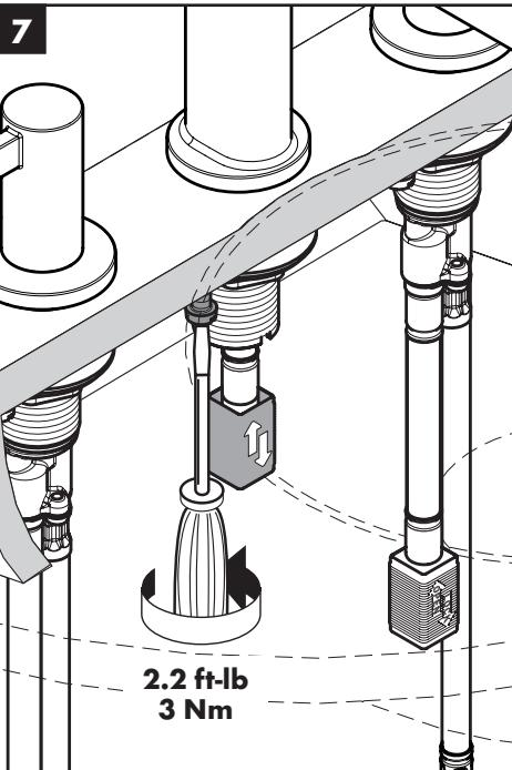
Tighten the tensioning screws.
