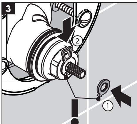
\*\*To prevent scald injury, the maximum output temperature of the shower valve must be no higher than 120°F (49°C). In Massachusetts, the maximum output temperature can be no higher than 112°F (44°C).
