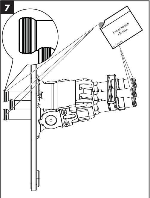
Lightly lubricate the O-rings on the swivel unit using white plumber's grease.
