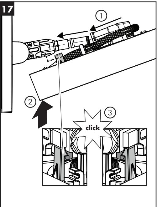
Push the inlet of the showerhead over the supply tubes, then push upward so that the clips on the showerhead engage the swivel unit.
