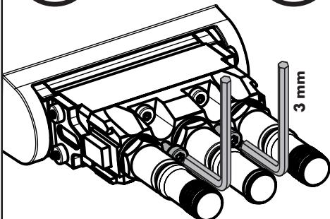
If the tension is too loose, tighten the tension screws on the swivel unit using a 3mm Allen wrench.
