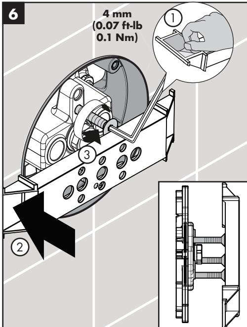
Remove the backing from the adhesive on the fitting aid.
