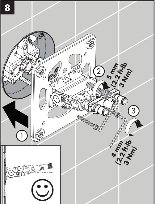
Install the M8x45 cylinder screw using a 5 mm Allen wrench. Install the two M5x40 cylinder screws using a 4 mm Allen wrench.
