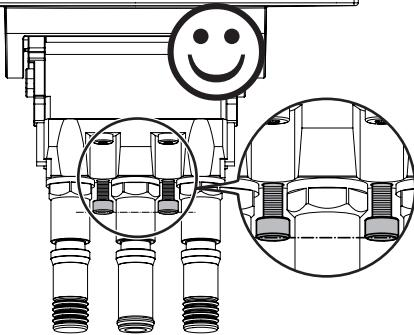
⚠ Make sure that the tension screws are tightened evenly.
