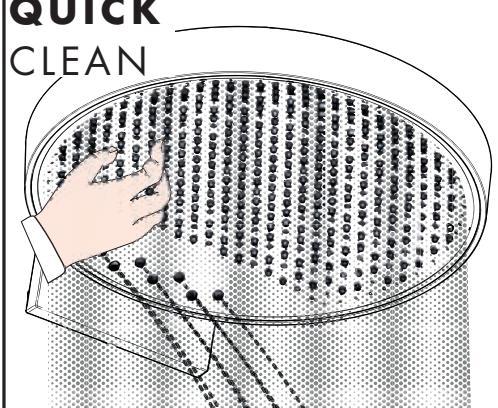
**Just clean:** simply rub over the spray nozzles to remove lime scale.
