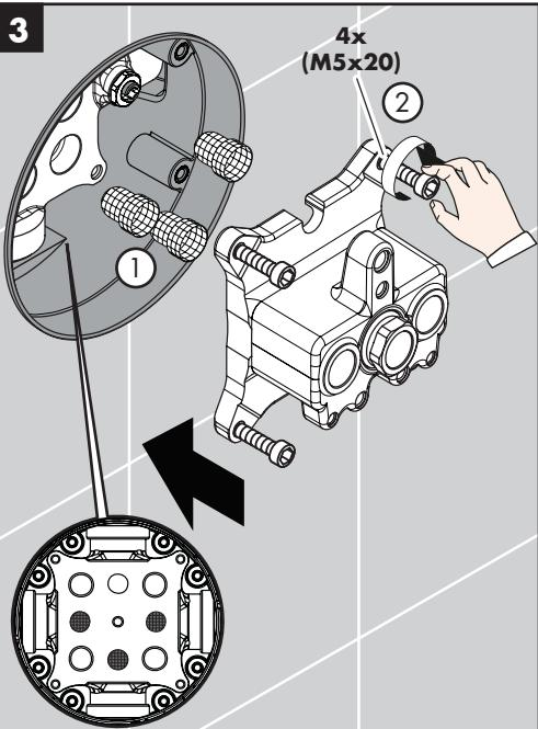
Install the filters in the left, right, and bottom inlets on the iBox.
