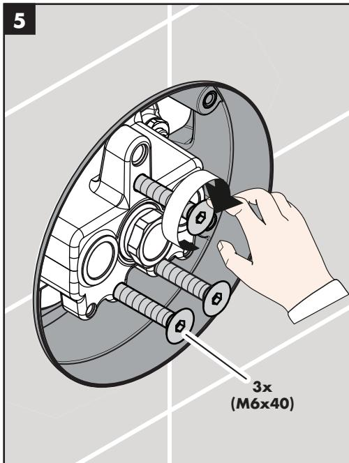
Install the three M6x40 countersunk screws by hand.
