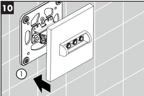
Push the escutcheon over the swivel unit and against the wall.
