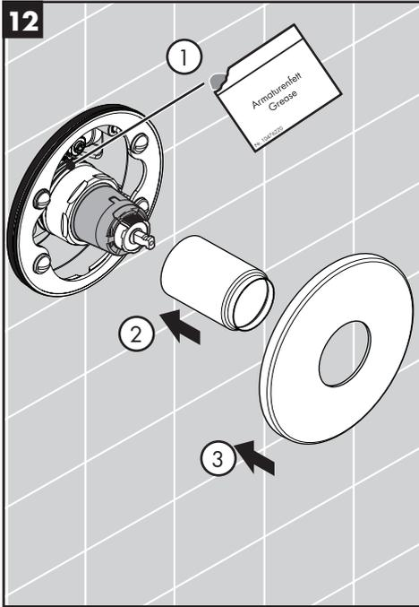
Lubricate the cartridge o-ring using a small amount of white plumber's grease.
