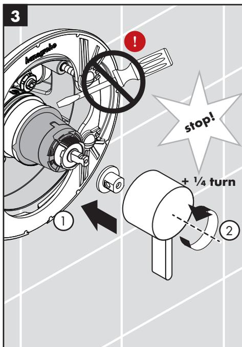
⚠ **Do not attempt to pry the cartridge from the function block by using a screwdriver as doing so can damage the cartridge. Damage to the cartridge can result in property damage.**
