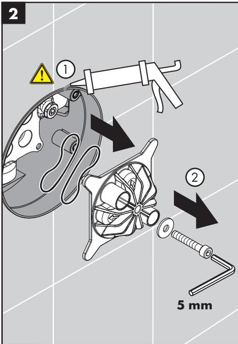
Seal the wall around the plaster shield with water-proof sealant.
