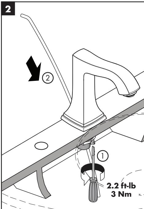
Tighten the tensioning screws.
