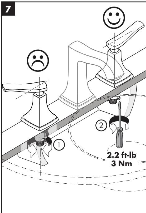
If it is unsatisfactory, loosen the tensioning screw.
