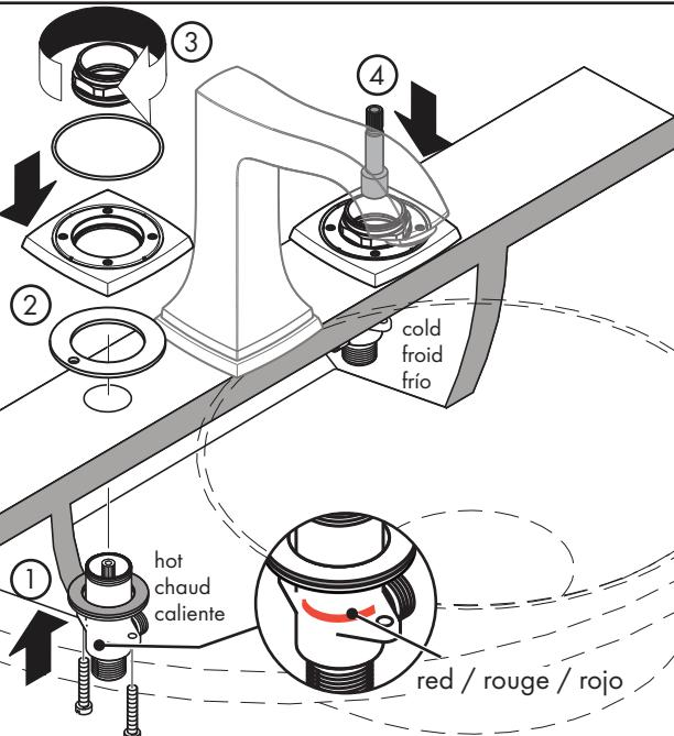
Push the hot and cold valves up through the mounting surface.
