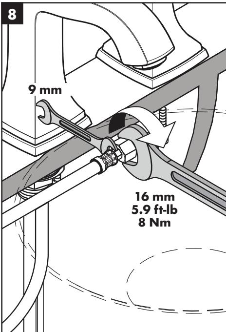
Connect the spout hoses to the hot and cold valves.
