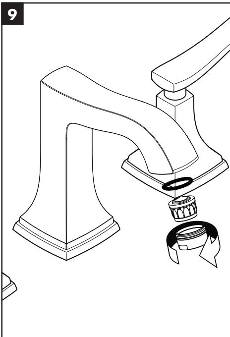
Remove the aerator using a 22 mm wrench.
