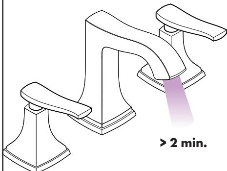
Turn the water on. Allow the faucet to flush for at least two minutes.
