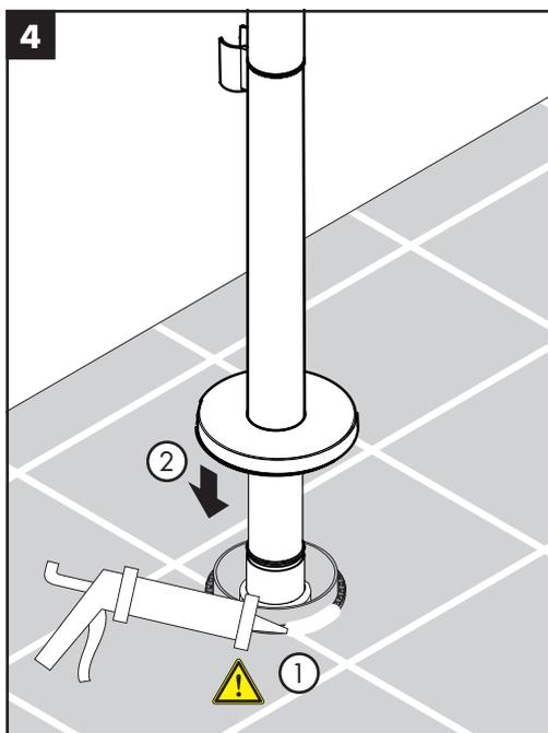
**Seal the floor around the plaster shield with waterproof sealant.**
