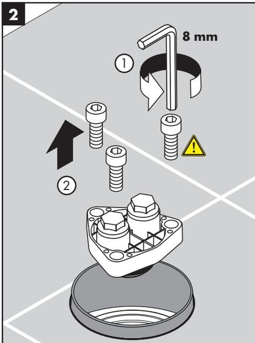
Remove the flush housing screws.
