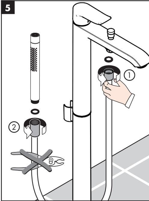
Place the black rubber washer in the short hose end. Attach this end to the tub filler.
