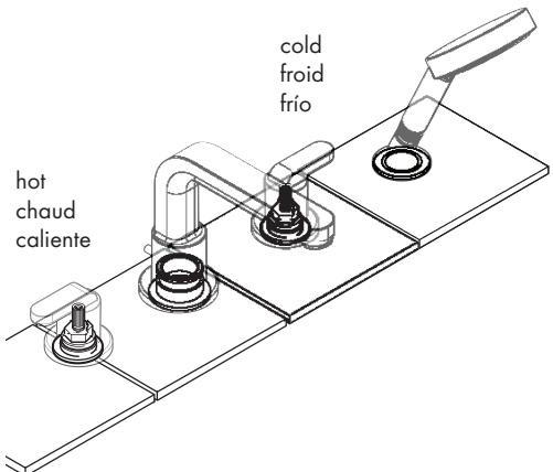
**⚠ To insure correct operation of the faucet, install the hot supply on the left and the cold supply on the right.**
