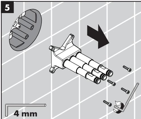
Remove the pipe assembly.
