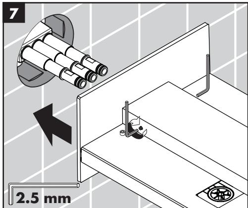
Push the Rainfall over the pipe assembly and against the wall.
