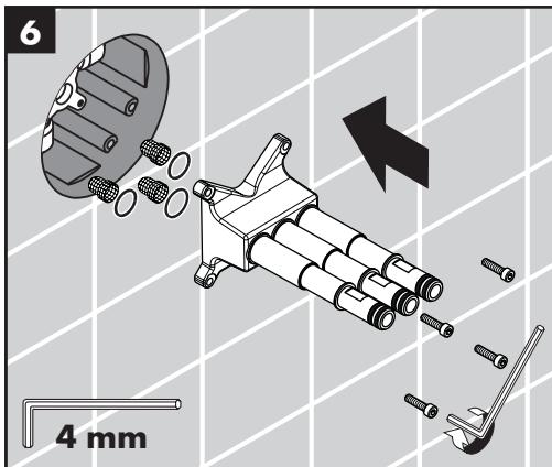
Install the filters, seals, and pipe assembly.
