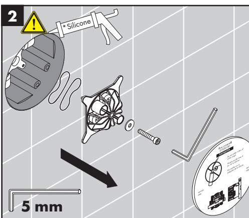
Remove the cover, flush insert, and seal.
