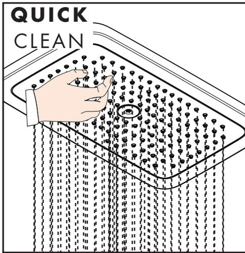
**EN** Just clean: simply rub over the spray nozzles to remove lime scale.
