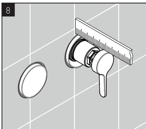
Measure the distance from the wall to the top of the handle.
