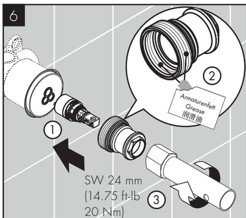
Insert the cartridge and the seal.
