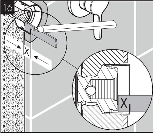
Measure the distance between the outside edge of the spout plaster shield and the spout housing ("X").
