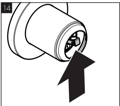
Push the cartridge stem upward.
