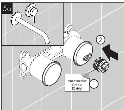
Lightly lubricate the o-ring on the cartridge adapter.
