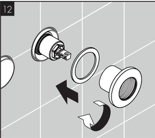
Install the seal and the handle escutcheon.
