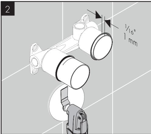
Cut the plaster shields so that they extend 1/16" (1 mm) beyond the surface of the finished wall.
