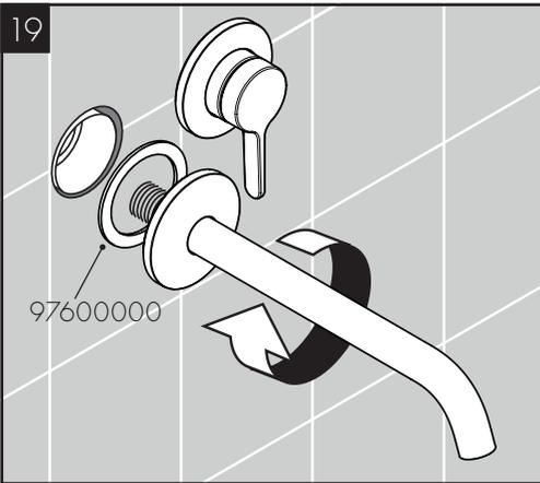
Install the sealing ring and the spout.
