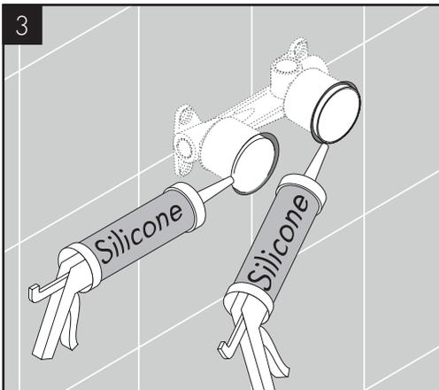
Seal the wall around the plaster shields using waterproof sealant.
