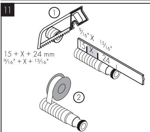
Add  $1\frac{1}{2}$ " (39 mm) to X. Cut the spout connecting thread so that it is  $X + 1\frac{1}{2}$ " ( $X + 39$  mm) long.
