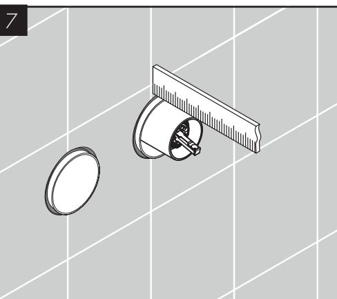
Measure the distance from the wall to the top of the nut.
