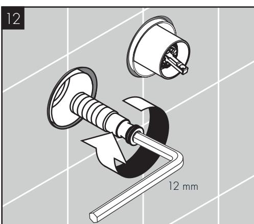
Install the connecting thread in the rough using a 12 mm Allen wrench.
