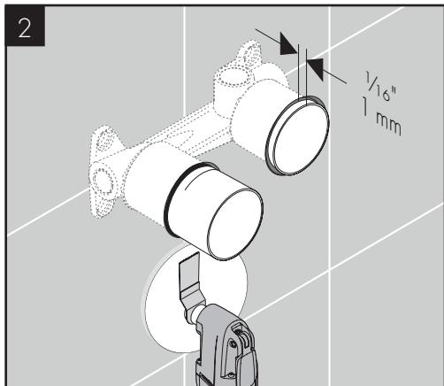
Cut the plaster shields so that they extend  $\frac{1}{16}$ " (1 mm) beyond the surface of the finished wall.
