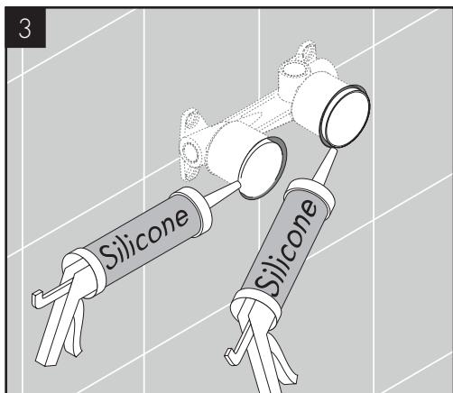
Seal the wall around the plaster shields using waterproof sealant.
