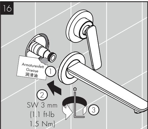
Lightly lubricate the o-ring on the connecting thread using plumber's grease.
