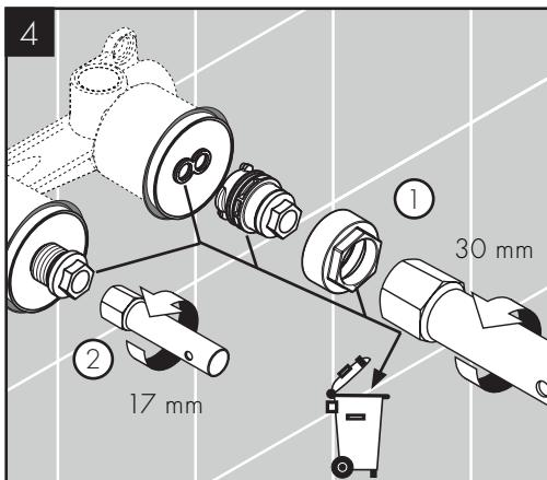
Remove the nut and the flush insert from the cartridge housing.
