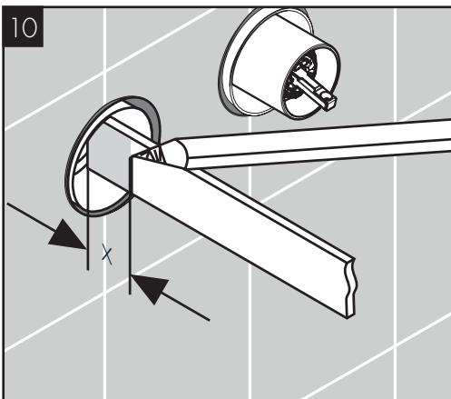
Measure the distance between the outside edge of the spout plaster shield and the spout housing ("X").
