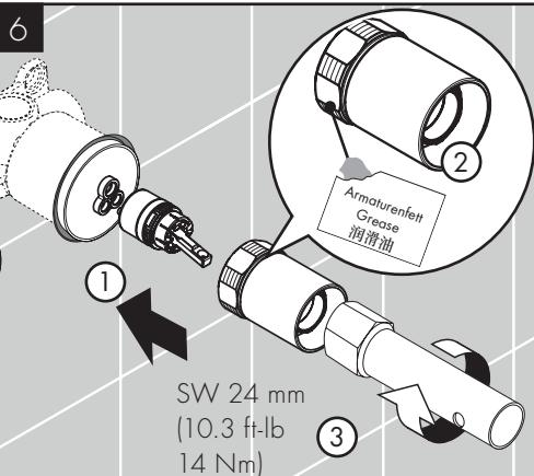
Insert the cartridge and the seal.
