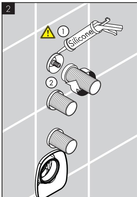
Seal the wall around the plaster shields using water-proof sealant.
