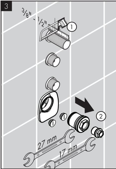
Cut the slip connector so that it extends  $\frac{3}{8}$ " -  $\frac{1}{2}$ " (10 - 13 mm) outside the surface of the finished wall.
