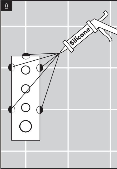
Place a dab of waterproof sealant on the wall at the grout joints.
