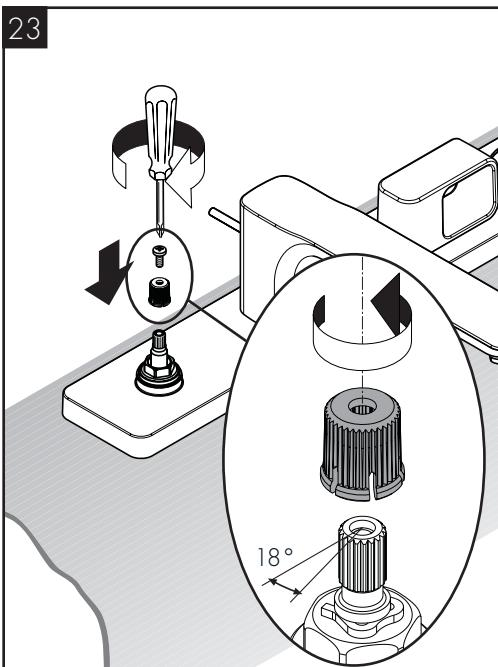
Rotate the snap connector slightly. Reinstall the snap connector and screw.
