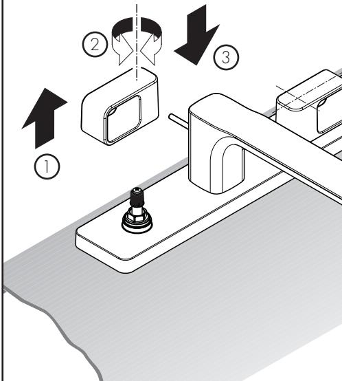
Remove, rotate, and reinstall the handle(s).
