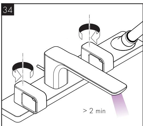
Flush the hot and cold supplies for a minimum of two minutes.
