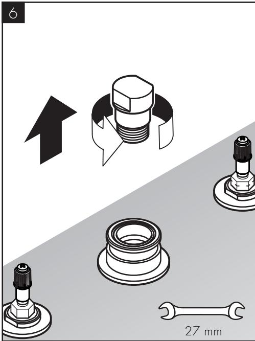
Remove the plug from the diverter housing.
