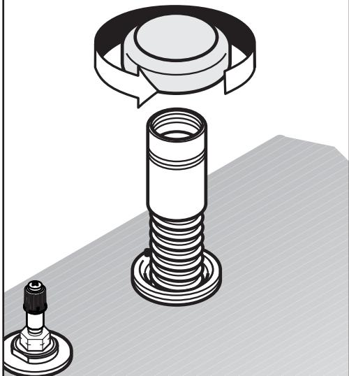
Remove the plaster shield from the Secuflex hose.
