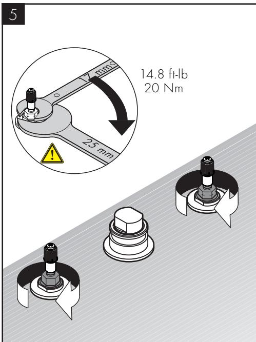
Tighten the new cartridge using two wrenches.
