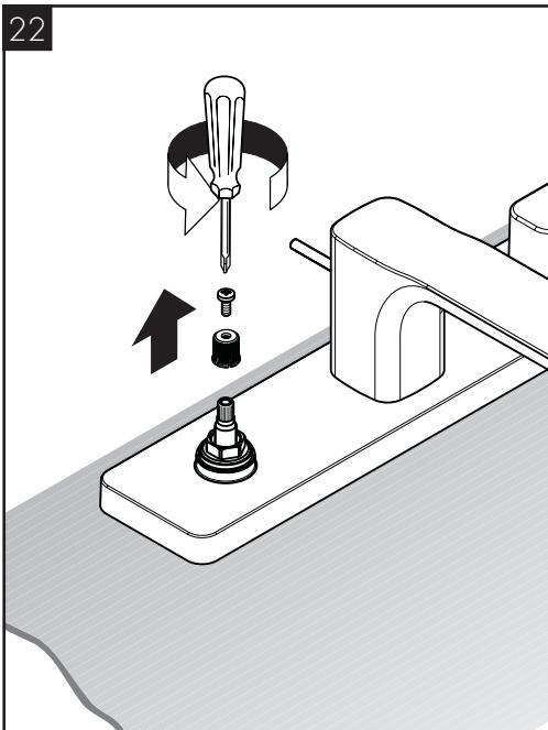
Remove the snap connector and screw.
