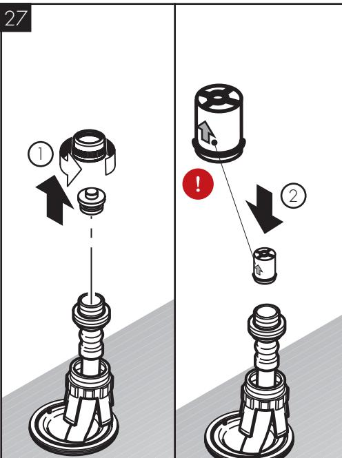
Remove the brass plug and nut.
