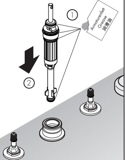
Lightly lubricate the o-rings on the diverter using white plumbers grease.
