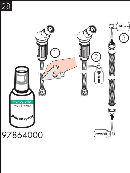
Lubricate the handshower hose using silicone spray.
