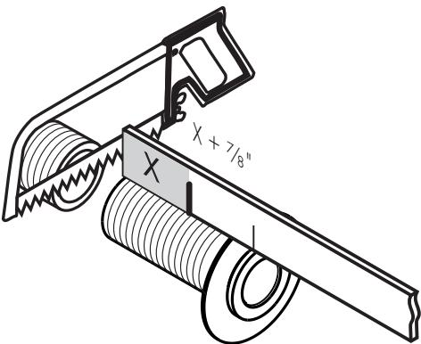
Cut the mounting nipple so that it is  $X + \frac{7}{8}$ " ( $X+23$  mm) long.
