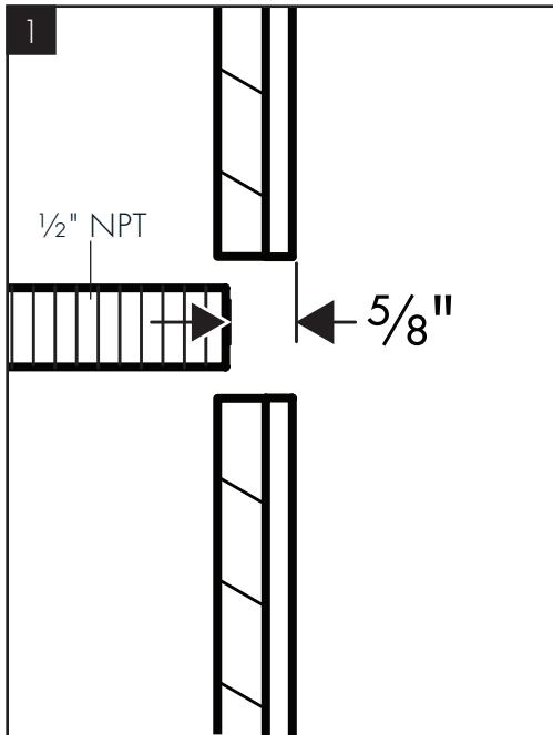
⚠ This installation requires a  $\frac{1}{2}$ " NPT male nipple, recessed  $\frac{5}{8}$ " behind the surface of the finished wall.
