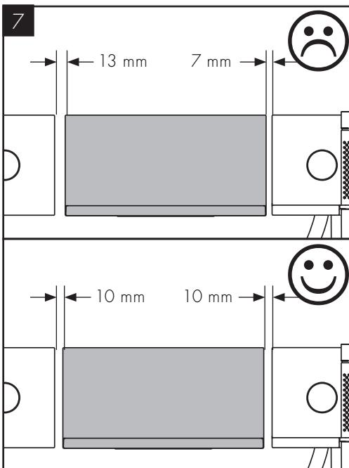
If using in a manifold installation, make sure that the spout is centered between the other two components.
