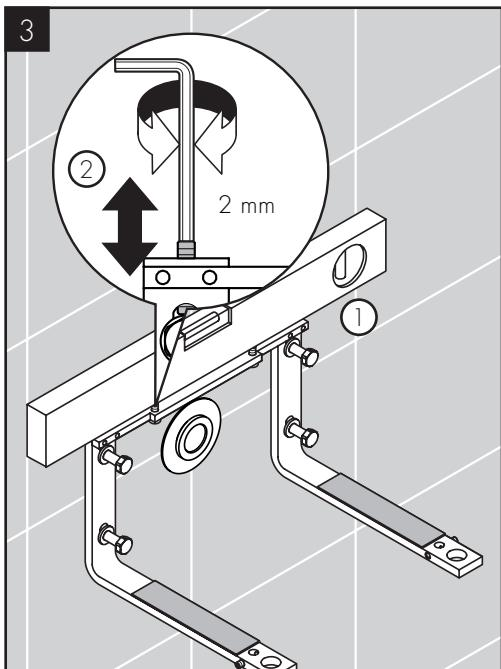
Make sure that the mounting frame is level. Use a 2 mm Allen wrench to raise or lower the leveling screws.
