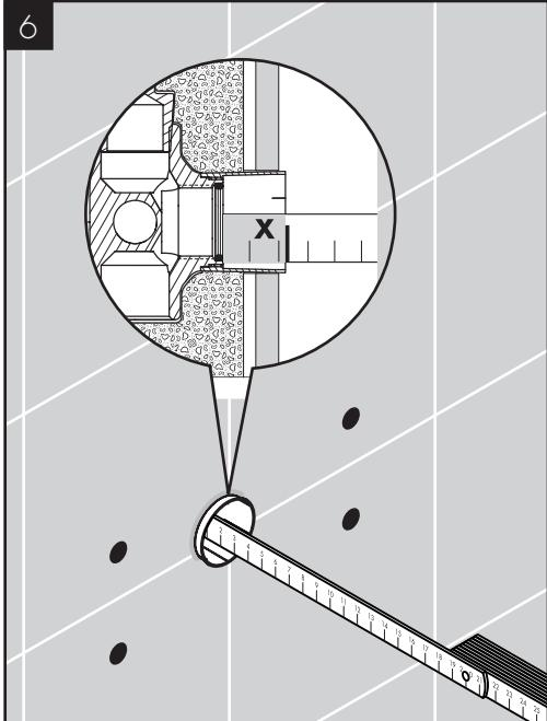
Measure the distance from the edge of the plaster shield to the brass part of the rough (X).
