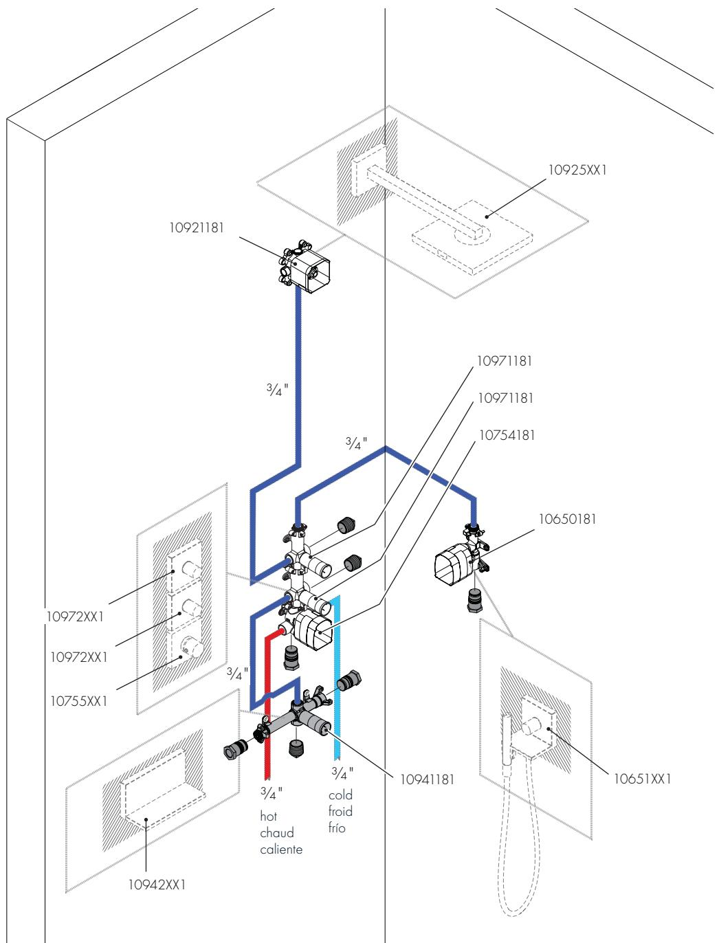
INSTALLATION WITH ROUGH 10941181 / INSTALLATION AVEC PIÈCE INTERIEURE
