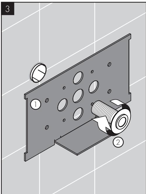
Install the template. Install the mounting piece
