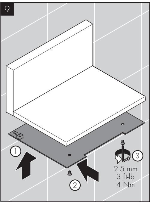
Install the base plate. Tighten the screws using a 2.5 mm Allen wrench.
