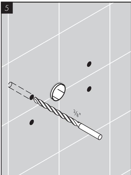
Drill the holes using a  $\frac{3}{8}$ " (8 mm) bit.
