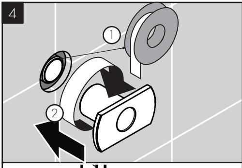
Wrap the threads on the nipple using plumbers' tape.
