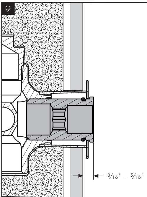
The mounting piece should extend  $\frac{3}{16}$ " -  $\frac{5}{16}$ " outside the surface of the finished wall.
