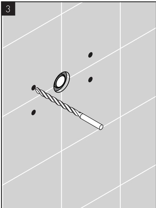
Drill the holes using an  $\frac{3}{8}$ " (8 mm) bit.
