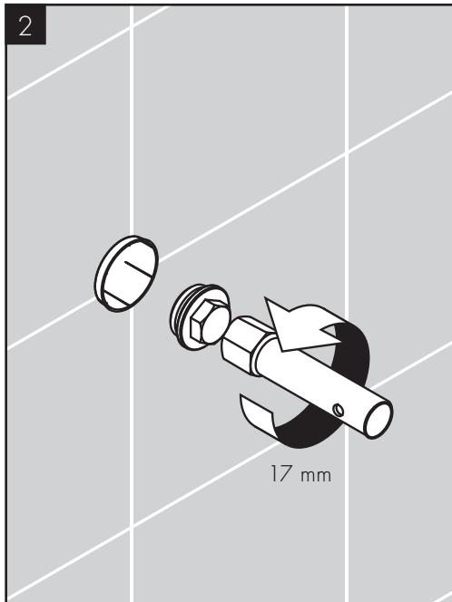
Remove the plug using a 17 mm wrench..
