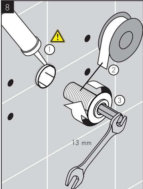
$\triangle$  Seal the wall around the plaster shield using waterproof sealant.
