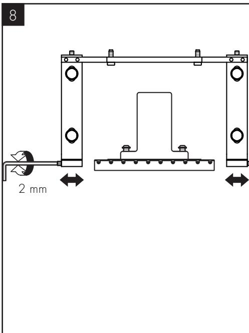
Use a 2 mm Allen wrench to adjust the centering screws.
