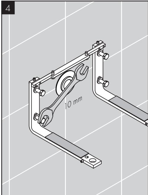
Tighten the screws using a 10 mm wrench.
