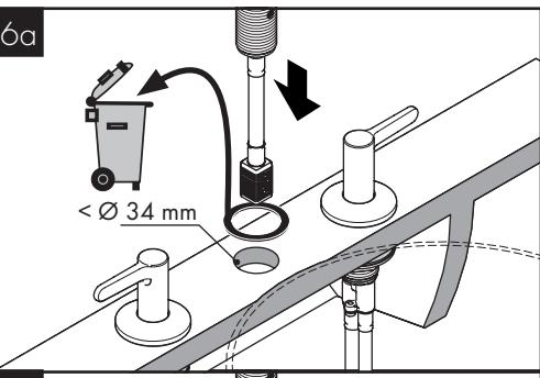
If the hole for the spout is less than  $1\frac{5}{16}$ " (34 mm), discard the sealing ring.
