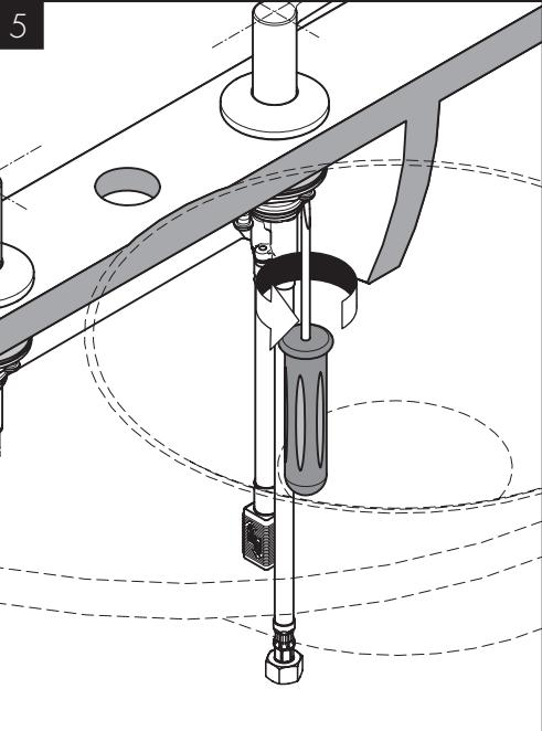
5 Tighten the nut. Tighten the tensioning screws.
