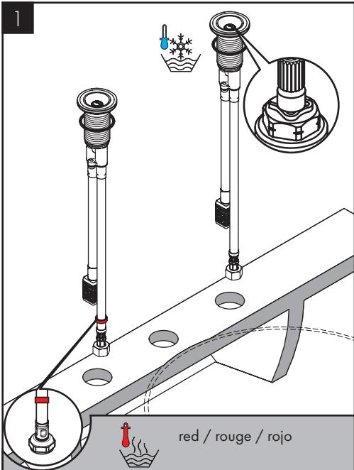
Place the hot and cold valve assemblies and the O-rings on the mounting surface. The hot valve should be on the left, the cold valve on the right.
