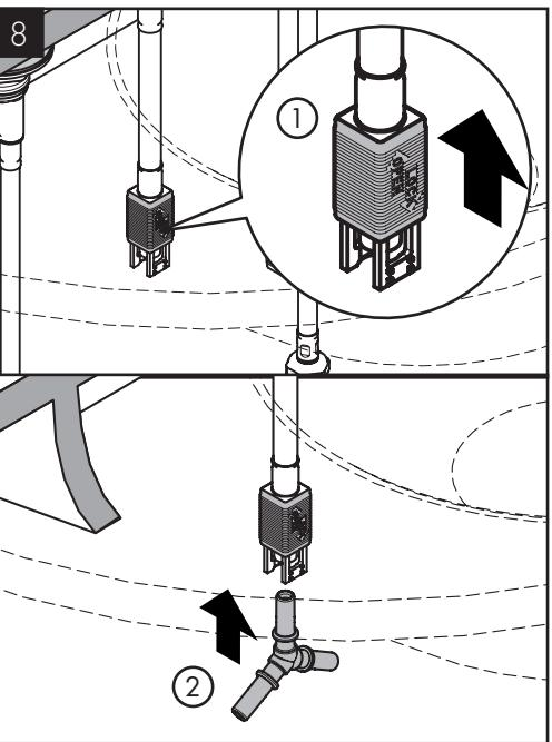
Open the quick-connect by pushing it upwards.
