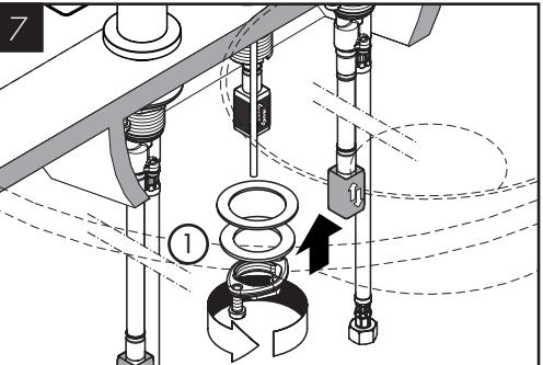
Install the fiber washer, metal washer, and mounting nut.
