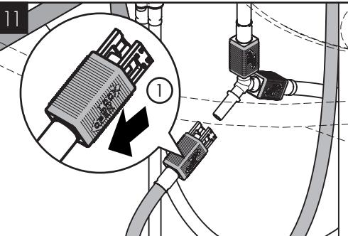
Open the quick-connect on one of the connection hoses by pushing it upwards.
