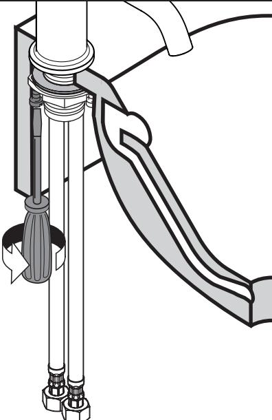
Tighten the tensioning screws using a screwdriver.
