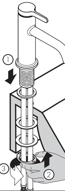
48210XX1 only: Install the drain pull rod.
