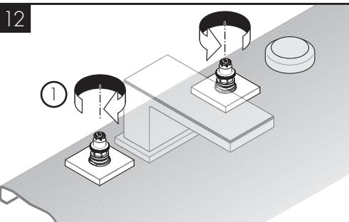
Rotate the cartridges to the closed position - clockwise on the cold side, counter-clockwise on the hot side.
