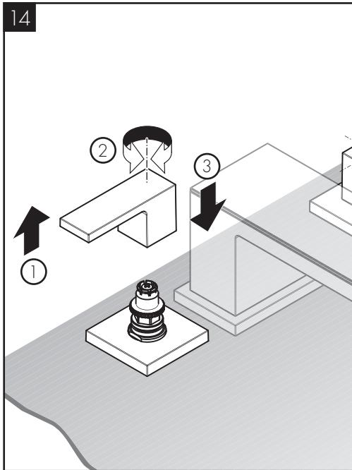
If necessary, remove, rotate, and reinstall the handles.
