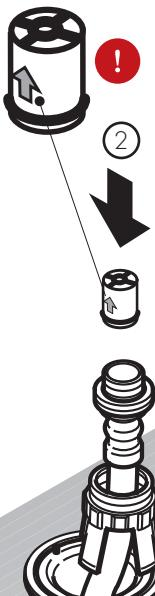
Remove the brass plug and nut from the high pressure hose. Install the check valve.
