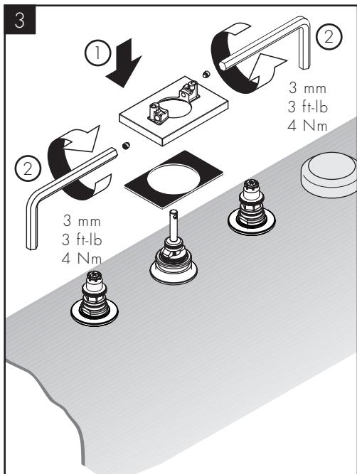
Push the seal and escutcheon over the diverter.
