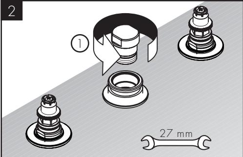
Remove the plug from the spout tee using a 27 mm wrench.
