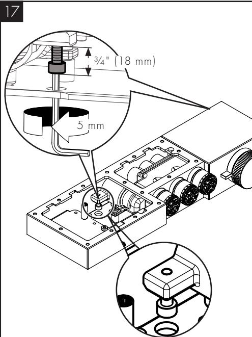
Use a 5 mm Allen wrench to loosen the two large retaining screws so that the ends of the screws extend  $\frac{3}{4}$ " (18 mm) below the flanges.
