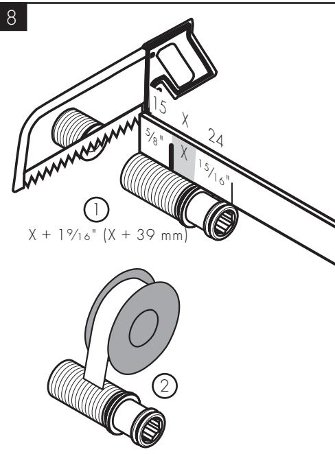
Cut the two manifold nipples so that they are  $X + 1\frac{9}{16}$ " ( $X + 39$  mm) long.
