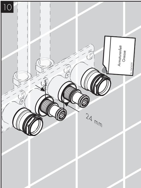
The manifold nipples should extend  $1\frac{5}{16}$ " (24 mm) beyond the edge of the plaster shield.
