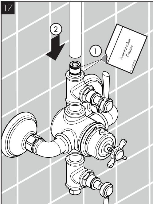
Lubricate the o-rings on the riser.
