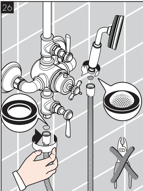
Place the black rubber hose washer in one end of the hose. Screw this end to the handshower port on the valve.
