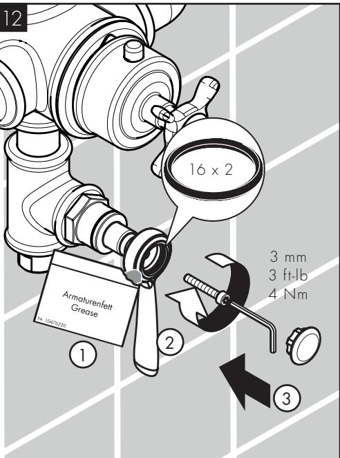
Lightly lubricate the handle o-ring using white plumber's grease.
