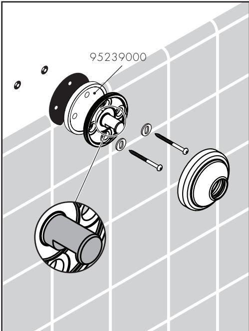
If the tile does not go all the way up the wall, install the mounting plate with the tile matching disk, #95239000 (not included).
