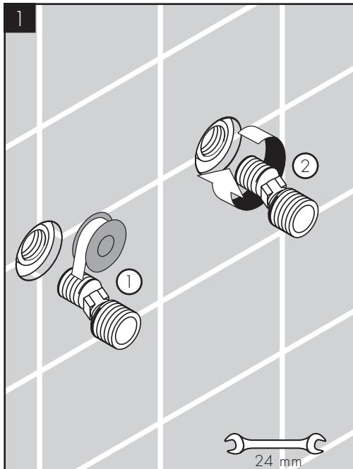
Wrap the threads on the NPT  $\frac{1}{2}$  side of the s-union with plumber's tape.
