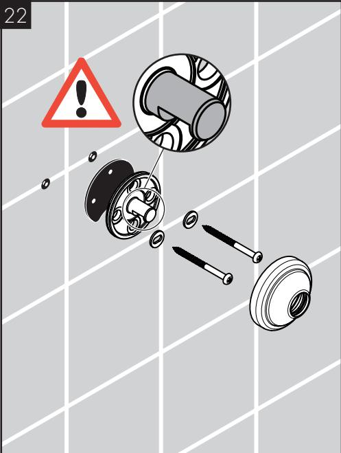
Install the shower arm mounting plate using the included screws and washers.
