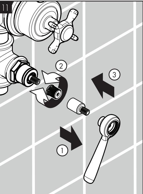
If it is still unsatisfactory, remove the handle, adapter, and snap connector.
