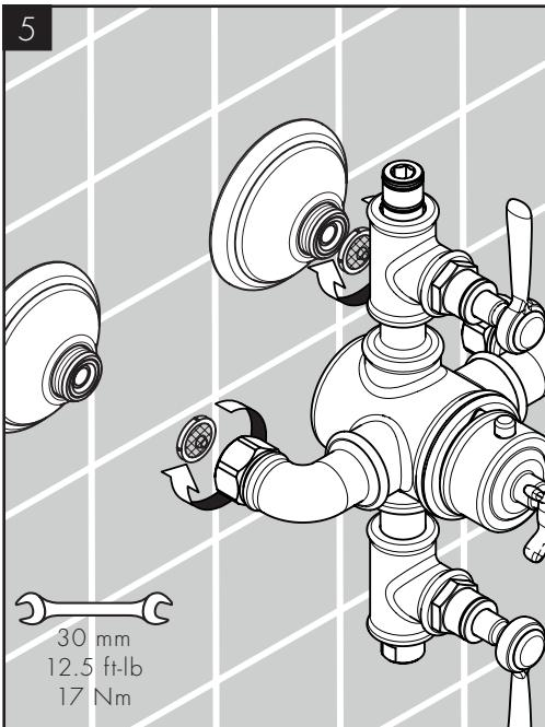
Connect the valve body to the s-unions. Do not over-tighten the nuts.
