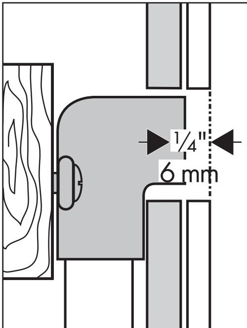
Install  $\frac{1}{2}$ " NPT female fittings, recessed  $\frac{1}{4}$ " (6 mm) behind the surface of the finished wall, for the hot and cold water supplies.
