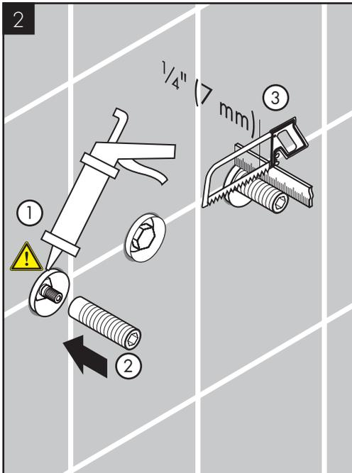
Seal the wall around the plaster shields with waterproof sealant.
