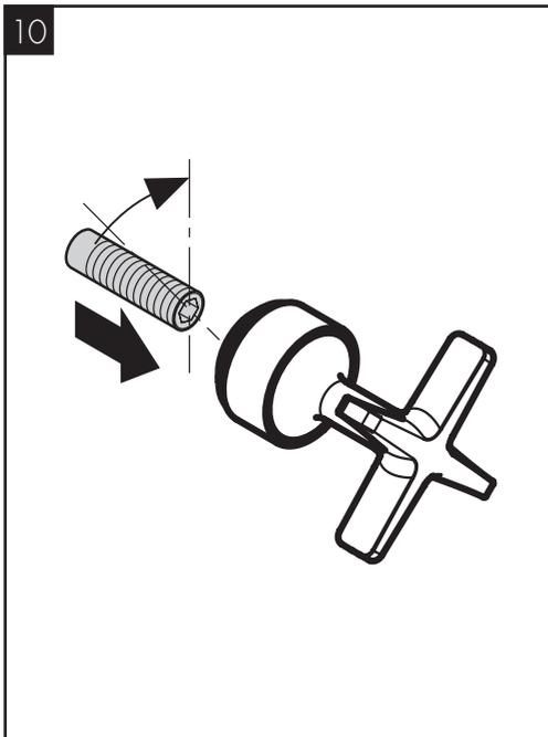
Remove, rotate, and reinstall the extension spindle.
