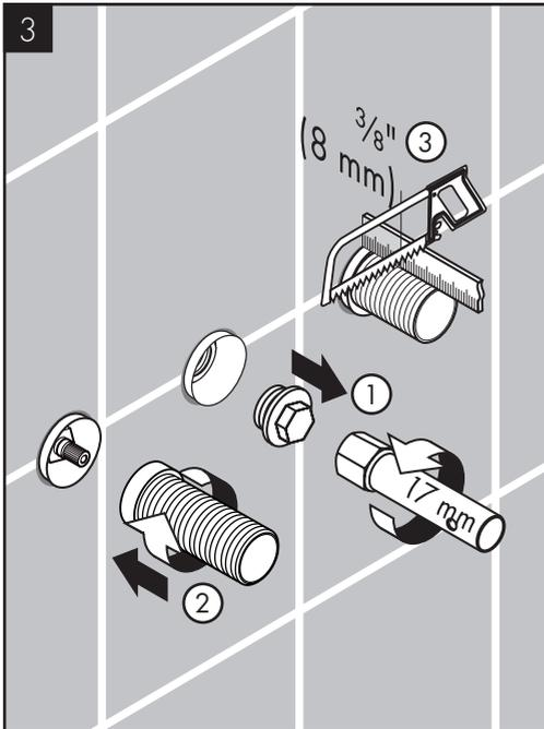
Remove the plug from the spout housing.
