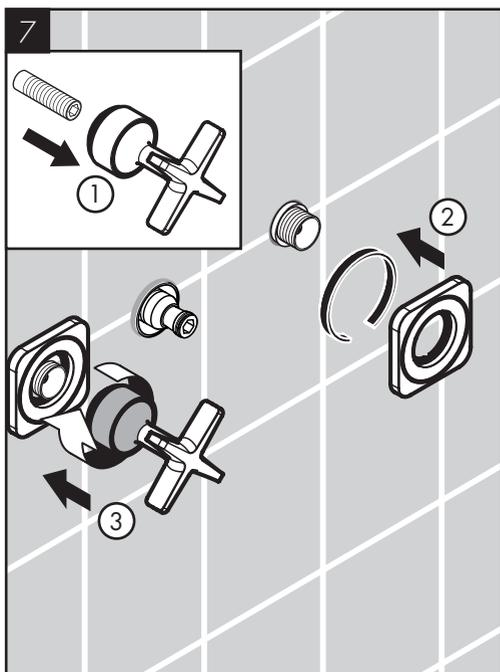
Insert the extension spindles in the handles.
