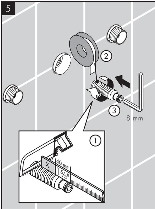
Cut the threaded end of the nipple so that it is  $1\frac{5}{8}'' + X$  (40 mm + X) long.
