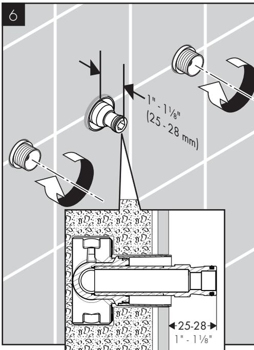
The nipple should extend  $1'' - 1\frac{1}{8}''$  (25 - 28 mm) from the surface of the finished wall.
