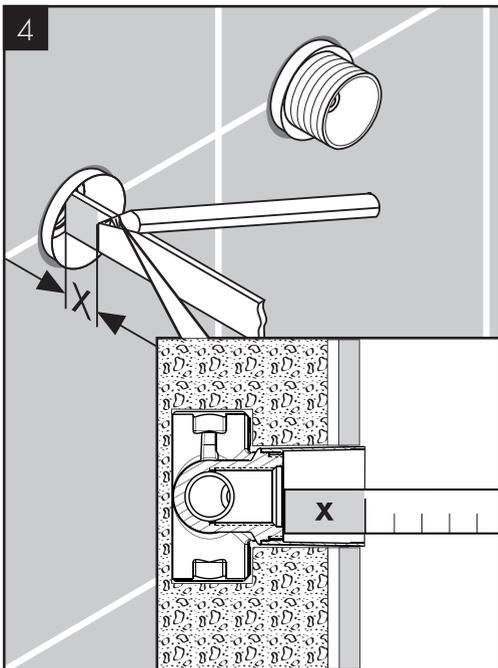
Measure the distance between the front of the spout housing and the surface of the wall. Record this measurement ("X").
