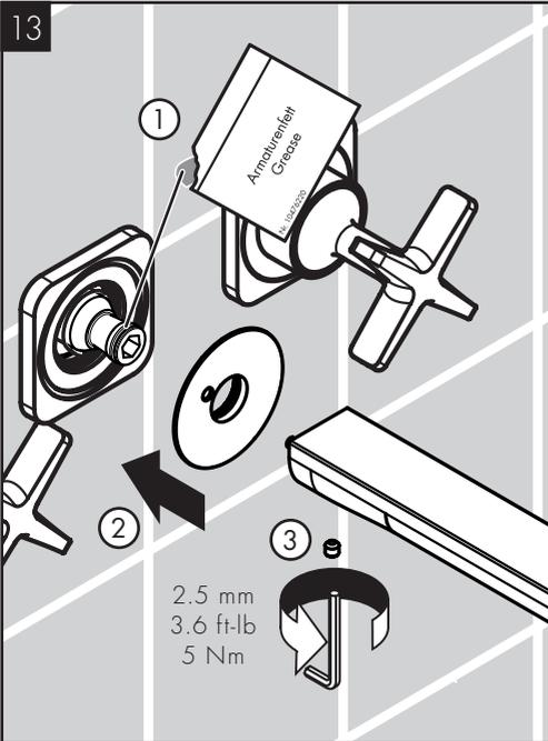
Lightly lubricate the nipple o-ring.
