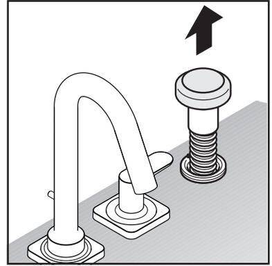
Lubricate the o-rings with silicon spray.
