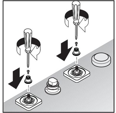
Make sure that the valve stems are in the off position.
