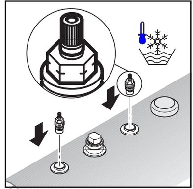
Hold the valve steady with a 25 mm wrench while tightening the cartridge with a 17 mm wrench.
