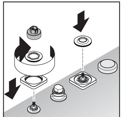
Install the handle snap connectors on the valve stems.
