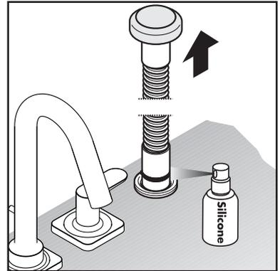
Pull the Secuflex hose out until the white plastic nut clears the mounting surface and the metal high pressure hose can be grasped (1).
