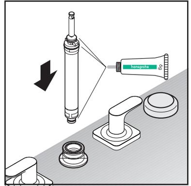
Place the sealing ring, escutcheon, and flange over the diverter stem.
