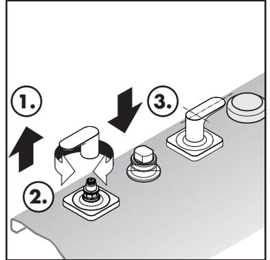
Remove the spout tee plug using a 27 mm wrench.
