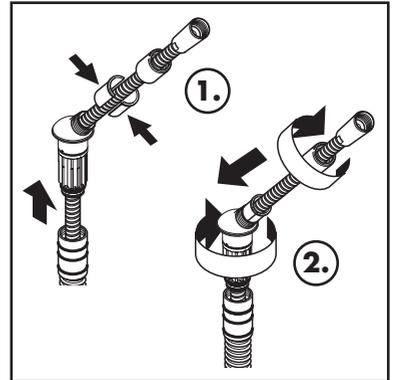
Remove the o-rings from the bottom of the Secuflex hose.
