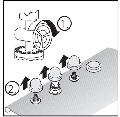
Remove the hot and cold cartridges from the rough. Hold the valve still with a 25 mm wrench while unscrewing the cartridge with a 17 mm wrench.
