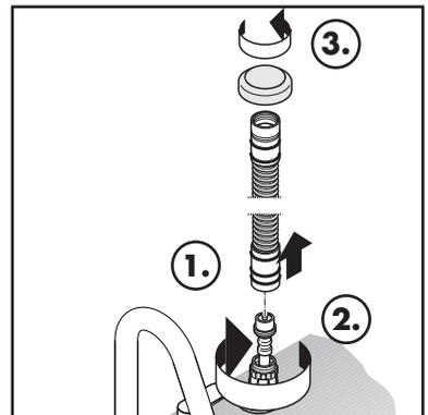
Remove the plug from the end of the high pressure hose (1).
