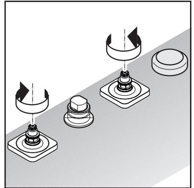
Position the handle and color ring over the stem. Press
