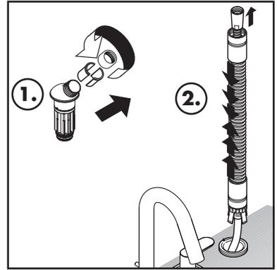
Feed the handshower hose through the handshower holder. Snap the two halves of the insert around the hose. Slide the nut over the end of the hose (1).
