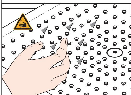
EN / Important! Components with damaged surfaces must be exchanged, otherwise there could be an injury danger.
