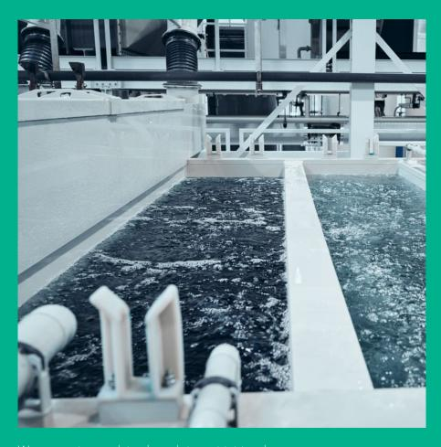
Wastewater is reused in electroplating, minimizing the amount of wastewater. The removed metals such as copper nickel, and chrome are recycled.
