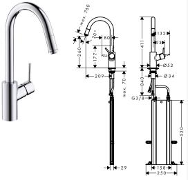
**Talis M52** Single lever kitchen mixer 260, installation in front of a window, pull-out spout, 1 jet, sBox
