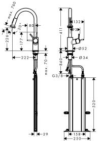
Talis M52 Single lever kitchen mixer 220, installation in front of a window, pull-out spray, 2jet, sBox
