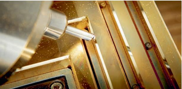
RIGHT: A line that will become a diamond cut in the finished appearance is milled up to five times. LEFT, TOP AND BOTTOM: A diamond is used to mill the beveled chamfer at an angle of exactly 45° to a high gloss.
