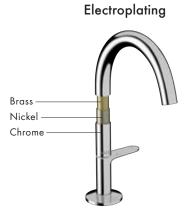
Chrome is the standard surface in the sanitary environment and has proven itself in the bathroom over many decades. Through the electrochemical deposition of various metals, and depending on the type of substrate, a copper layer is built up in the electroplating bath, followed by a bright nickel and chrome layer on the basic brass body.
