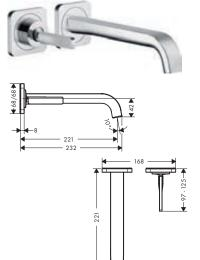
/ maximum flow rate at 3 bar: 5 l/min
