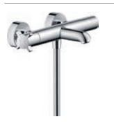
/ flow rate of hand shower at 3 bar: 17 l/min / min. operating pressure: 1 bar / max. operating pressure: 10 bar / Safety stop at 40 °C / temperature limitation adjustable / non-return valve
