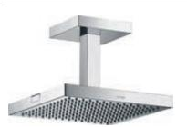
/ maximum flow rate at 3 bar: 12 l/min / flow rate RainAir spray (at 3 bar): 12 l/min / flow rate expansible to 25 l/min / minimum flow pressure: 2 bar / spray disc removable for cleaning / installation: ceiling
