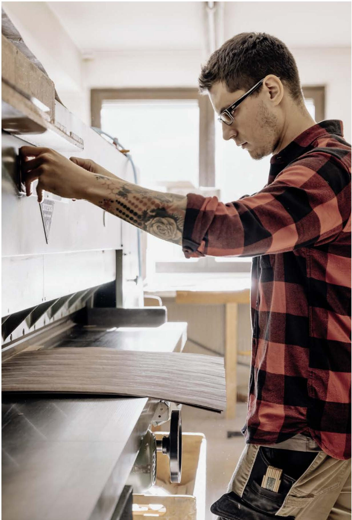
The veneer packets are pressed and cut to the dimensions of the final format. For additional stability, the wood panel on the back is precision-milled and glued to a stainless steel plate. A laser is used to apply the AXOR logo to the plate. Finally, the exposed veneer surface of the plate is oiled to protect the material and give it an elegant sheen.
