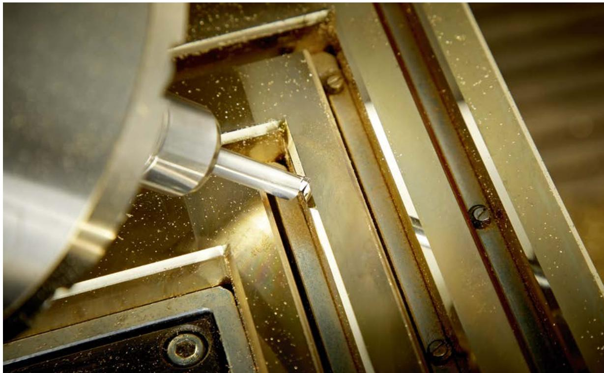
The chamfers are milled at an angle of exactly 45°.
