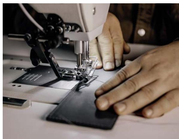
A majority of the processing is still done meticulously by hand. This includes the sewing of the cover plate and the applying of the AXOR logo with a hot stamp.
