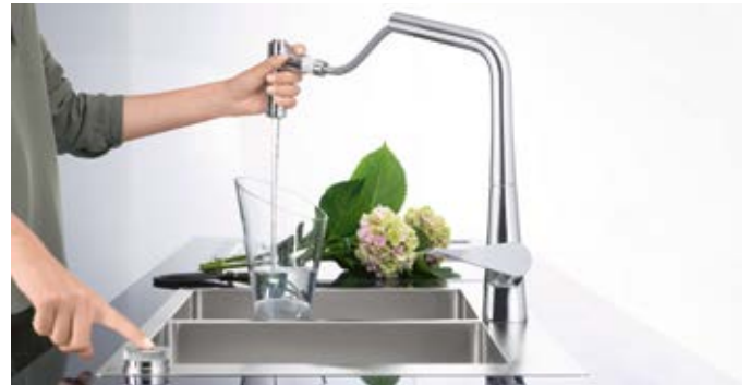
The hand spray expands the operating radius, while the hose is protected from damage as it is secured in the sBox. With the Select button at the front of the sink, the water can be turned on and off at the touch of a button. The handle remains open, maintaining water volume and temperature.
