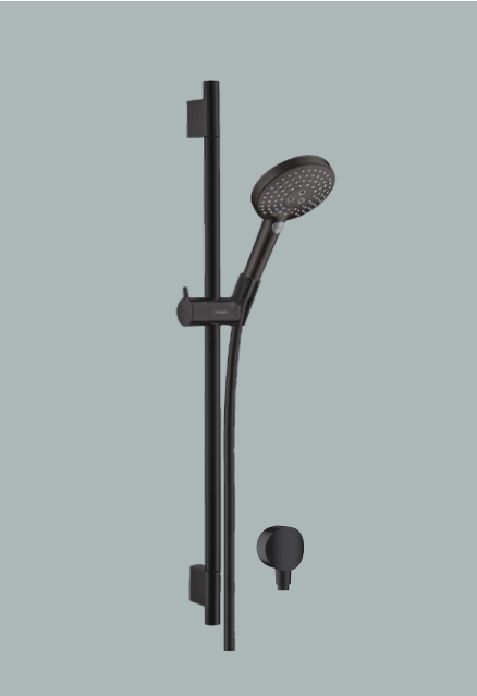
Raindance Select S Shower set 120 3jet EcoSmart 9 l/ min with shower bar 65 cm Required Parts # 28632670 Unica S Puro shower bar 65cm with hose # 26531670 Raindance Select S hand shower 120 3 jet # 26453670 FixFit S with non return valve # 93276000 Hose connection elbow (not shown) WELS 3 Stars, 9 l/min S07195
