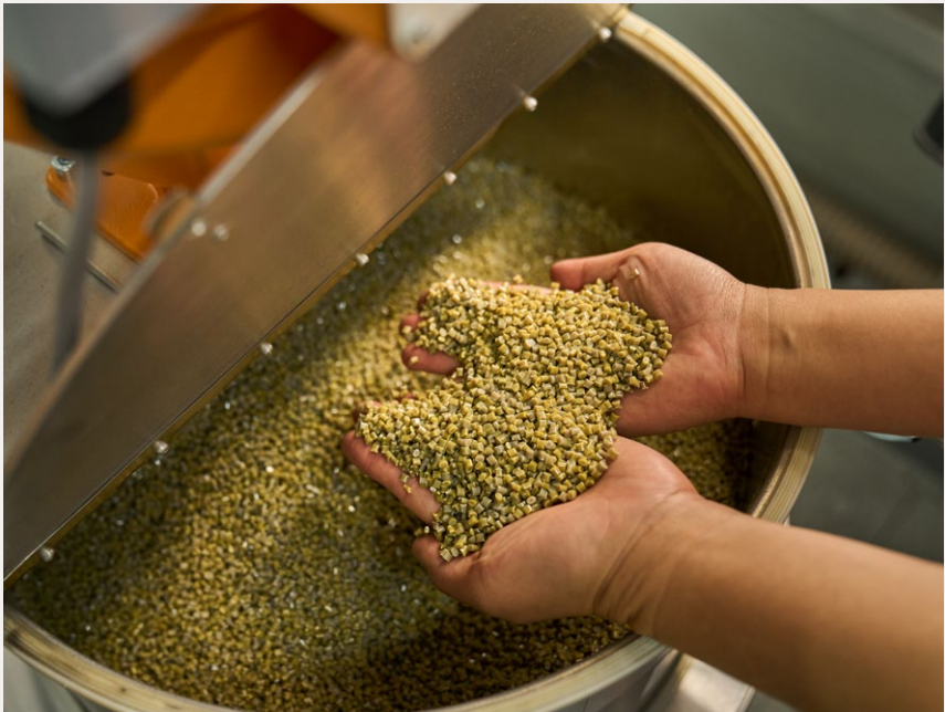
The recycled plastic pellets recovered from the processing plant are reintroduced into the cycle for the manufacture of new parts.
