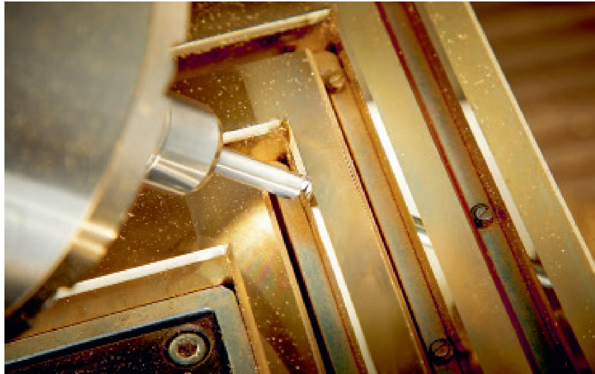
The chamfers are milled at an angle of exactly 45°.
