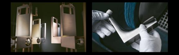
AXOR FinishPlus PVD surface finishes have character. and refined in AXOR's vacuum chambers using the PVD (physical vapor deposition) process. An electric arc discharges in the high vacuum, gases combine with zirconium. The mixture hits the faucet's chrome surface. This high-tech process gives the surface unprecedented brilliance and high resistance to scratches, cleaning agents, and the salt of the sea air.
