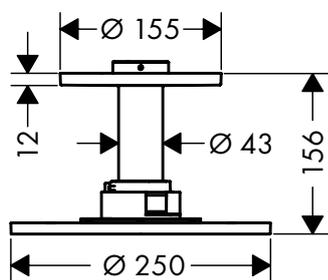
Thermostatic module for concealed installation for 3 functions
