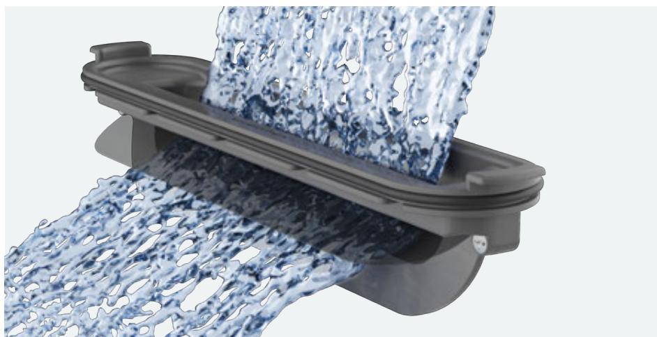
The innovative Dryphon siphon solution is included with every pre-fab set (RainDrain) of the drainage channels and, on request, can replace the supplied siphon of the uBox universal (basic set) and its drain performance of up to 42 l/min. The patented design offers a significant improvement in drain performance, of up to 60 l/min. Thanks to the high flow rate, dirt and hair cannot stick, which reduces cleaning to a minimum.
