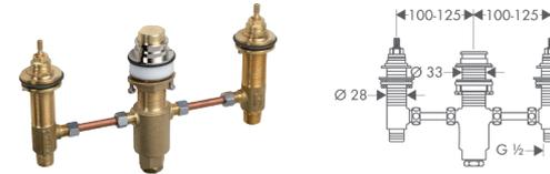
Technical drawing of a three-hole side-mount faucet base kit with dimensions: 100-125, 100-125, max. 40, 28, 33, G 1/2.
