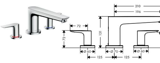
Technical drawing of a three-hole side-mount double-lever shower faucet with dimensions: 210, 196, 72, 131, 72, 109, 125, 125, 125, 60, 70, 60, 30.
