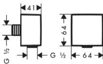
**Fixfit E 型软管墙面连接件, DN15**
