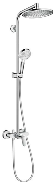
Crometta® S 240 Showerpipe with Crometta S 240 overhead shower, Crometta Vario hand shower and single lever mixer, shower arm 350 mm # 27269, -000
